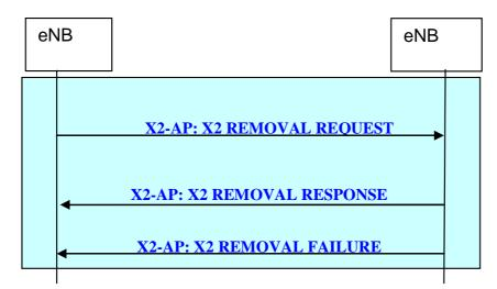
Figure 20.2.2.18-1: X2 Removal procedure
