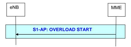
Figure 19.2.2.12.1-1 Overload Start procedure
