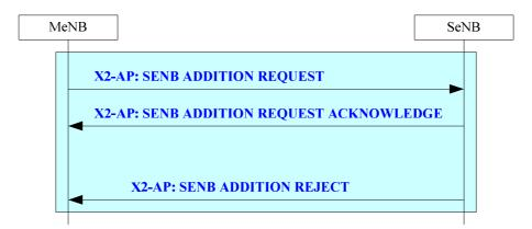
Figure 20.2.2.2a-1: SeNB Addition Preparation procedure
