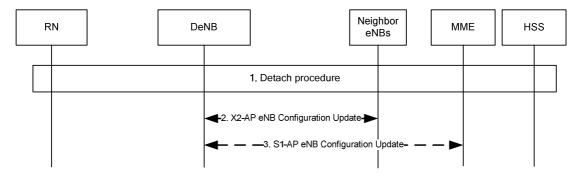
Figure 4.7.6.4-1: RN detach procedure
