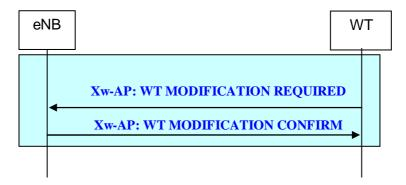
Figure 22B.2.2.4-1: WT initiated WT Modification procedure
