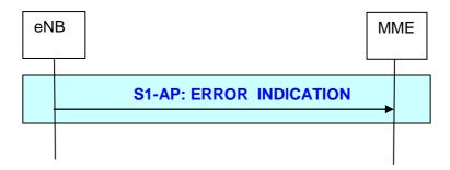
Figure 19.2.2.7.2a-1: eNB initiated Error Indication procedure
