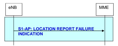
Figure 19.2.2.11.3-1: Location Report Failure Indication procedure
