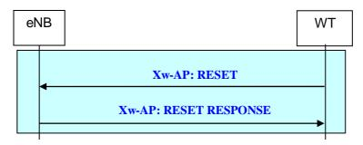
Figure 22B.2.2.12.1-1: Reset procedure initiated by WT
