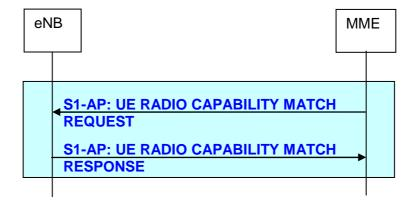
Figure 19.2.2.21-1: UE Radio Capability Match procedure
