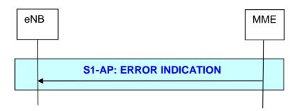
Figure 19.2.2.7.2b-1: MME initiated Error Indication procedure
