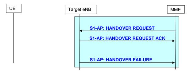
Figure 19.2.2.5.2-1: Handover resource allocation procedure
