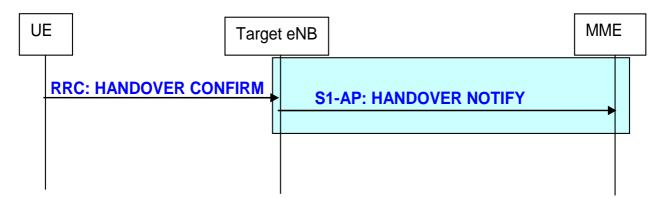
Figure 19.2.2.5.3-1: Handover completion procedure
