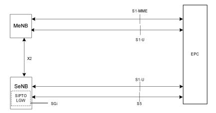
Figure 4.9.3.4-2: SIPTO@LN with co-located L-GW in SeNB
