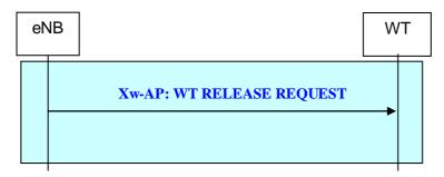
Figure 22B.2.2.5-1: eNB initiated WT Release procedure
