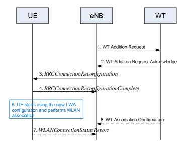
Figure 22A.1.7.1-1: WT Addition procedure
