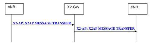
Figure 20.2.2.17-1: X2AP Message Transfer procedure
