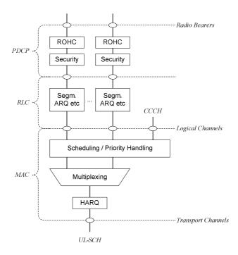
Figure 6-2: Layer 2 Structure for UL
