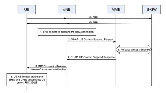
Figure 7.3a.3-1: RRC Connection Suspend procedure
