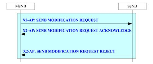
Figure 20.2.2.2c-1: MeNB initiated SeNB Modification Preparation procedure
