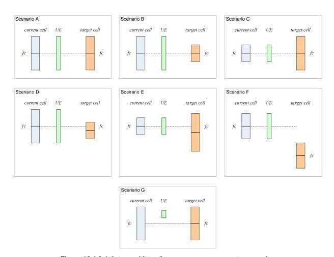
Figure 10.1.3-1: Inter and Intra-frequency measurements scenarios
