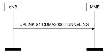
Figure 19.2.2.16.2-1: Uplink S1 CDMA2000 Tunnelling procedure
