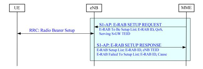
Figure 19.2.2.4.1-1: E-RAB Setup procedure
