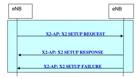
Figure 20.2.2.7-1: X2 Setup procedure
