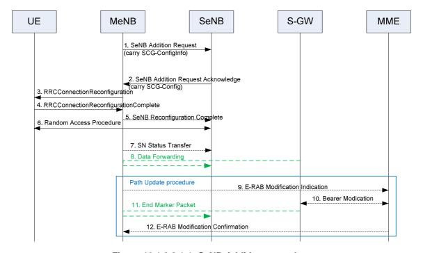
Figure 10.1.2.8.1-1: SeNB Addition procedure
