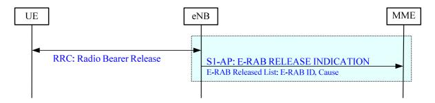
Figure 19.2.2.4.4-1: E-RAB Release Indication procedure
