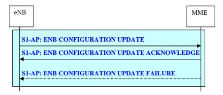
Figure 19.2.2.9-1: eNB Configuration Update procedure
