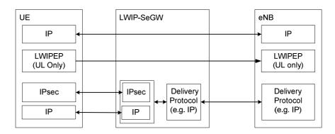
Figure 22A.3-3: Bearer over LWIP Tunnel - Protocol Stack
