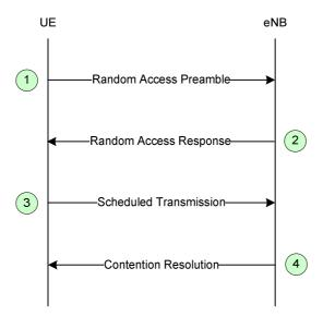
Figure 10.1.5.1-1: Contention based Random Access Procedure
