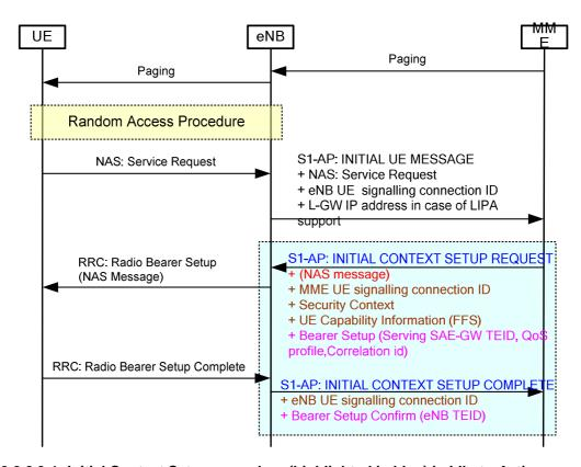
Figure 19.2.2.3-1: Initial Context Setup procedure (highlighted in blue) in Idle-to-Active procedure
