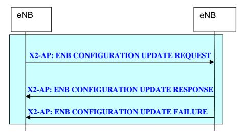
Figure 20.2.2.8-1: eNB Configuration Update procedure
