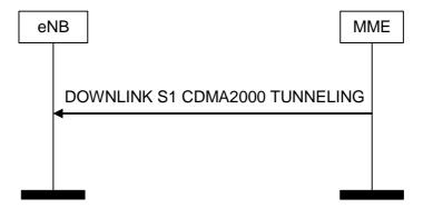
Figure 19.2.2.16.1-1: Downlink S1 CDMA2000 Tunnelling procedure
