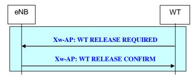
Figure 22B.2.2.6-1: WT initiated WT Release procedure
