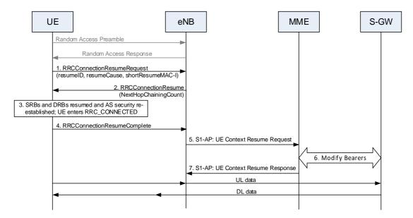
Figure 7.3a.3-2: RRC Connection Resume procedure
