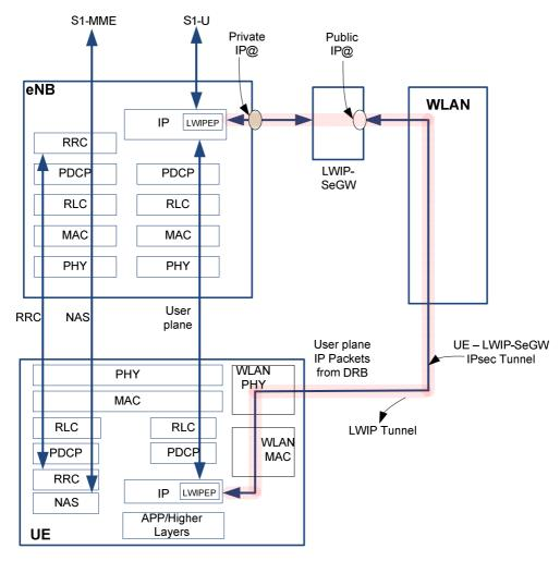
Figure 22A.3-2: LWIP Protocol Architecture
