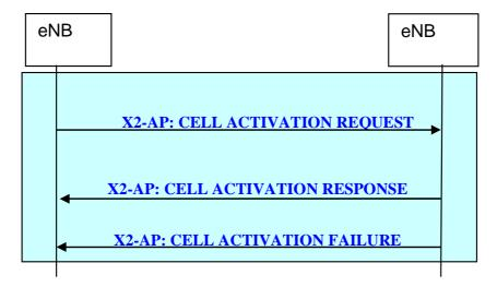
Figure 20.2.2.15-1: Cell Activation procedure
