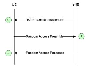
Figure 10.1.5.2-1: Non-contention based Random Access Procedure
