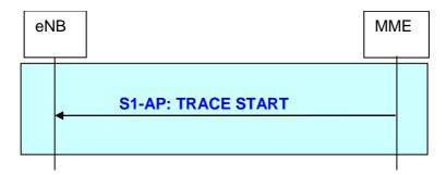
Figure 19.2.2.19.1-1: Trace Start procedure
