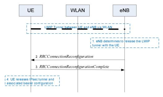
Figure 22A.3.1.3-1: LWIP tunnel release procedure
