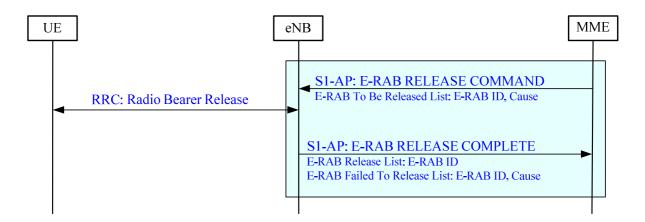
Figure 19.2.2.4.3-1: E-RAB Release procedure
