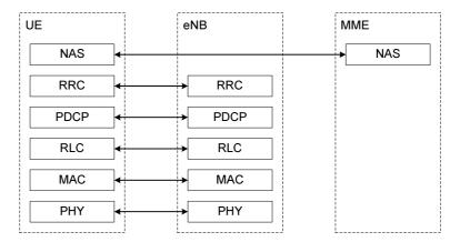
Figure 4.3.2-1: Control-plane protocol stack
