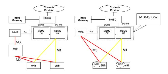
Figure 15.1.1-2: eMBMS Architecture deployment alternatives
