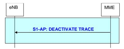
Figure 19.2.2.19.3-1: Deactivate Trace procedure
