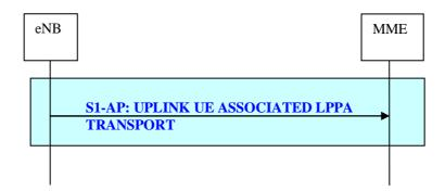
Figure 19.2.2.18.2-1: Uplink UE Associated LPPa Transport procedure
