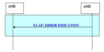
Figure 20.2.2.5-1: Error Indication procedure
