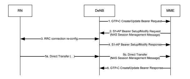
Figure 4.7.6.2-1: DeNB-initiated bearer activation/modification procedure
