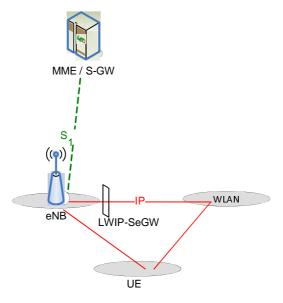
Figure 22A.3-1: LWIP Overall Architecture
