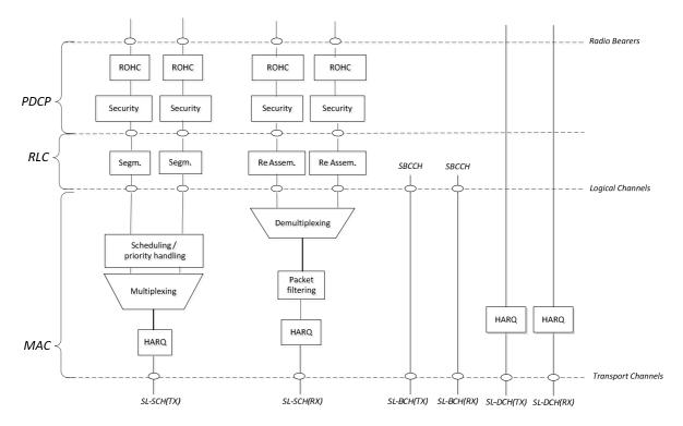
Figure 6-3: Layer 2 Structure for Sidelink
