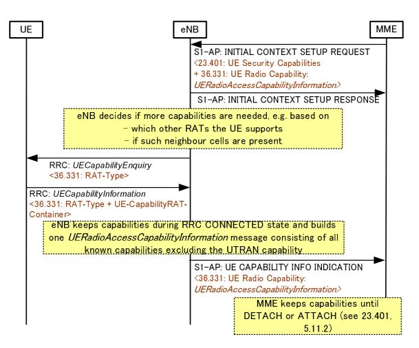
Figure 18-1: Initial UE Capability Handling
