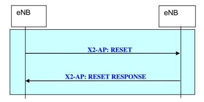
Figure 20.2.2.9-1: Reset procedure
