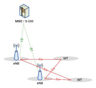
Figure 22A.1.1-1: Non-collocated LWA Overall Architecture
