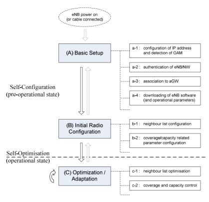
Figure 22.1-1: Ramifications of Self-Configuration /Self-Optimization functionality
