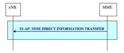
Figure 19.2.2.15-1: MME Direct Information Transfer procedure
