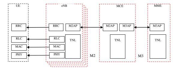
Figure 15.1.3-1: The E-MBMS c-plane architecture
