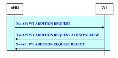
Figure 22B.2.2.1-1: WT Addition Preparation procedure
