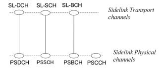
Figure 5.3.1-3: Mapping between sidelink transport channels and sidelink physical channels
