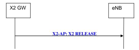
Figure 20.2.2.16-1: X2 Release procedure
