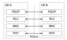
Figure 23.10.2.1-1: User-Plane protocol stack for sidelink communication
