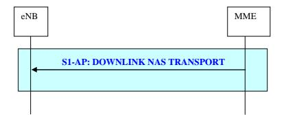
Figure 19.2.2.6-3: Downlink NAS Transport procedure
