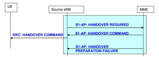
Figure 19.2.2.5.1-1: Handover preparation procedure
