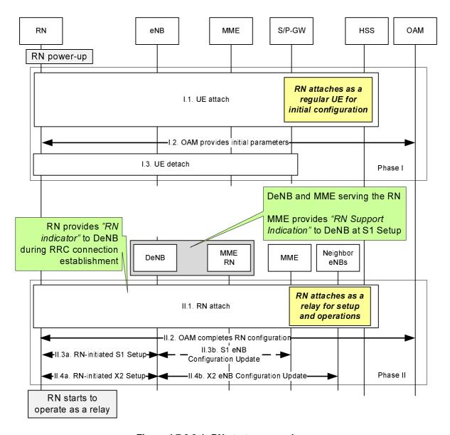
Figure 4.7.6.3-1: RN startup procedure
