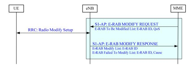
Figure 19.2.2.4.2-1: E-RAB Modification procedure
