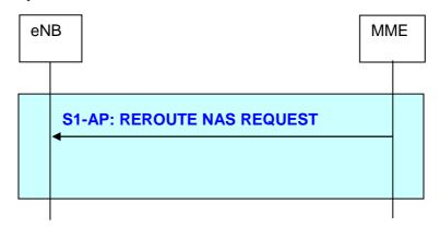
Figure 19.2.2.6-5: Reroute NAS Request procedure
