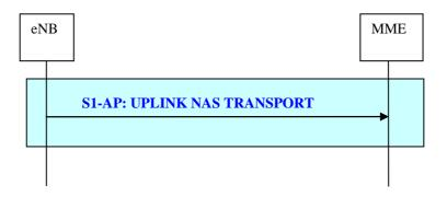
Figure 19.2.2.6-2: Uplink NAS Transport procedure
