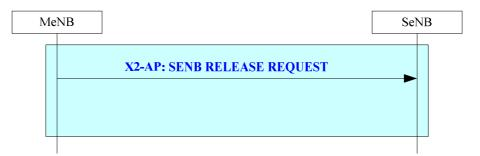
Figure 20.2.2.2e-1: MeNB initiated SeNB Release procedure
