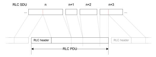
Figure 6.2.2-1: RLC PDU Structure
