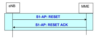
Figure 19.2.2.7.1a-1: eNB initiated Reset procedure
