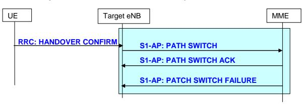
Figure 19.2.2.5.5-1: Path Switch procedure
