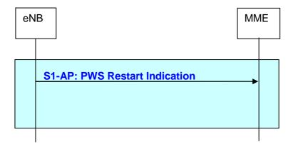
Figure 19.2.2.22-1: PWS Restart Indication procedure
