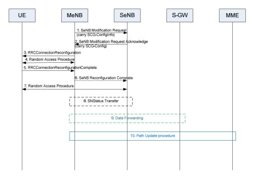
Figure 10.1.2.8.2.1-1: Intra-MeNB handover procedure with SeNB configuration
