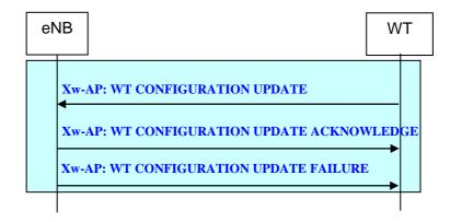
Figure 22B.2.2.10-1: WT Configuration Update procedure
