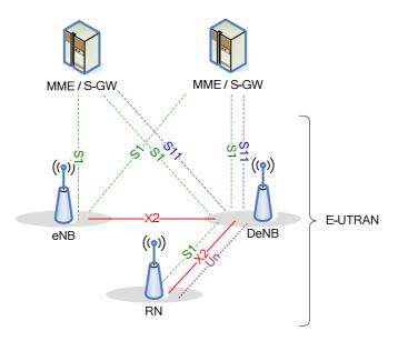
Figure 4.7.2-1: Overall E-UTRAN Architecture supporting RNs
