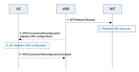
Figure 22A.1.7.3-1: WT Release procedure -eNB initiated
