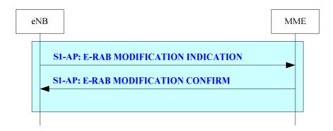
Figure 19.2.2.4.5-1: E-RAB Modification Indication procedure
