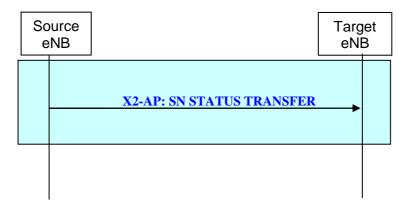
Figure 20.2.2.4-1: SN Status Transfer procedure
