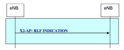
Figure 20.2.2.12-1: Radio Link Failure Indication procedure
