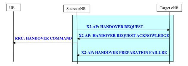
Figure 20.2.2.1-1: Handover Preparation procedure
