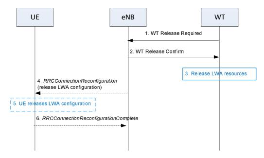
Figure 22A.1.7.3-2: WT Release procedure –WT initiated
