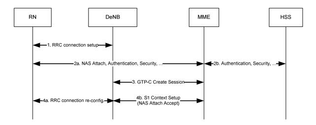
Figure 4.7.6.1-1: RN attach procedure
