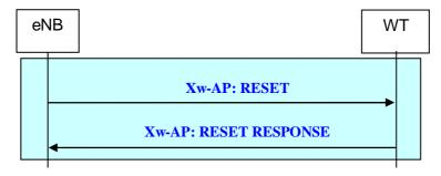
Figure 22B.2.2.12.2-1: Reset procedure initiated by eNB
