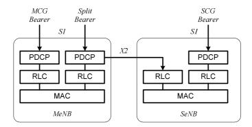
Figure 4.9.2-1: Radio Protocol Architecture for Dual Connectivity
