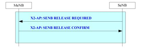
Figure 20.2.2.2f-1: SeNB initiated SeNB Release procedure
