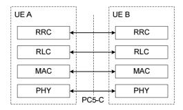
Figure 23.10.2.2-1: Control-Plane protocol stack for SBCCH
