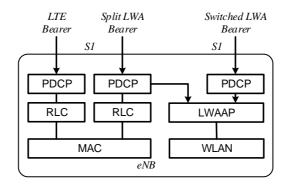
Figure 22A.1.2-1: LWA Radio Protocol Architecture for the Collocated Scenario
