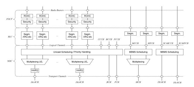
Figure 6-1: Layer 2 Structure for DL
