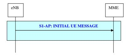
Figure 19.2.2.6-1: Initial UE Message procedure
