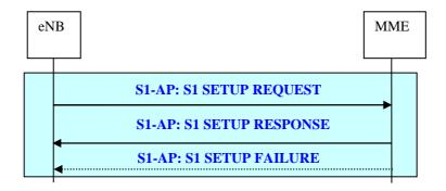
Figure 19.2.2.8-1: S1 Setup procedure
