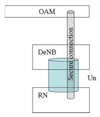
Figure 4.7.7.1-1: Relay OAM architecture.
