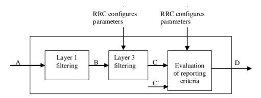
Figure 10.6-1: Measurement model
