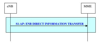
Figure 19.2.2.14-1: eNB Direct Information Transfer procedure
