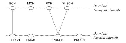
Figure 5.3.1-1: Mapping between downlink transport channels and downlink physical channels
