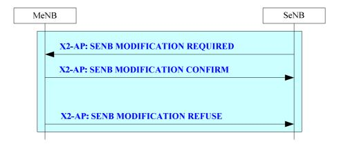
Figure 20.2.2.2d-1: SeNB initiated SeNB Modification procedure
