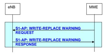
Figure 19.2.2.13.1-1: Write-Replace Warning procedure
