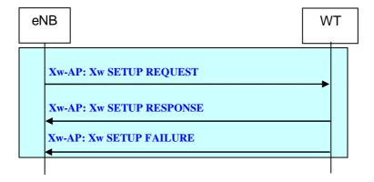
Figure 22B.2.2.9-1: Xw Setup procedure
