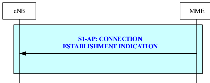
Figure 19.2.2.25-1: Connection Establishment Indication procedure
