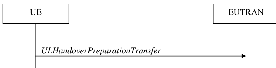
Figure 5.4.5.1-1: UL handover preparation transfer
