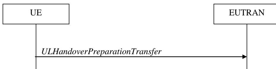
Figure 5.4.5.1-1: UL handover preparation transfer
