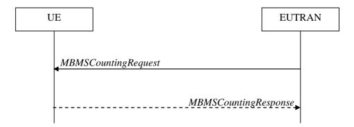
Figure 5.8.4.1-1: MBMS Counting procedure
