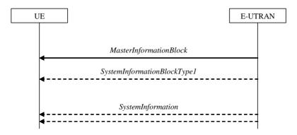
Figure 5.2.2.1-1: System information acquisition, normal
