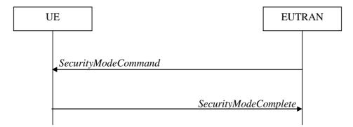
Figure 5.3.4.1-1: Security mode command, successful
