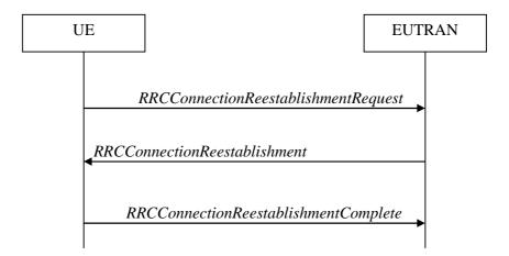
Figure 5.3.7.1-1: RRC connection re-establishment, successful
