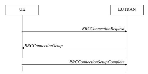
Figure 5.3.3.1-1: RRC connection establishment, successful
