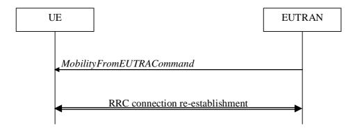
Figure 5.4.3.1-2: Mobility from E-UTRA, failure
