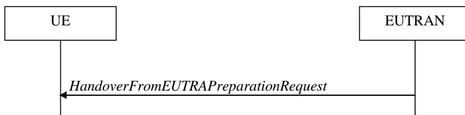
Figure 5.4.4.1-1: Handover from E-UTRA preparation request
