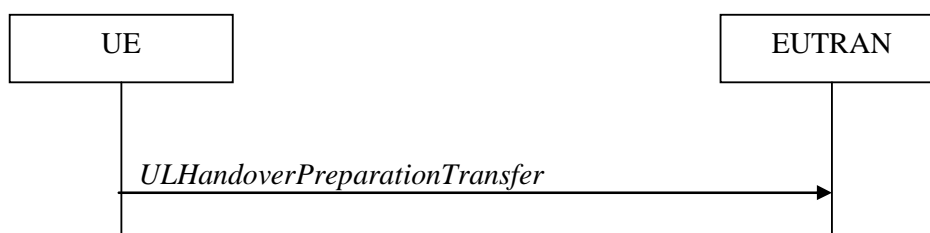
Figure 5.4.5.1-1: UL handover preparation transfer
