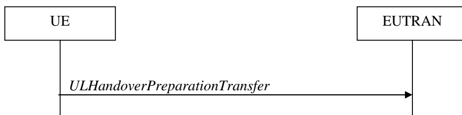
Figure 5.4.5.1-1: UL handover preparation transfer
