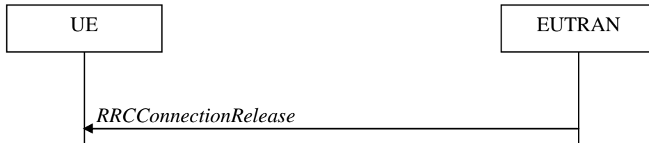
Figure 5.3.8.1-1: RRC connection release, successful
