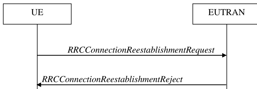
Figure 5.3.7.1-2: RRC connection re-establishment, failure
