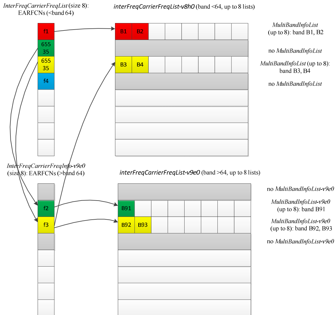
Figure D.1.2-1: Mapping of EARFCNs to MultiBandInfoList/MultiBandInfoList-v9e0
