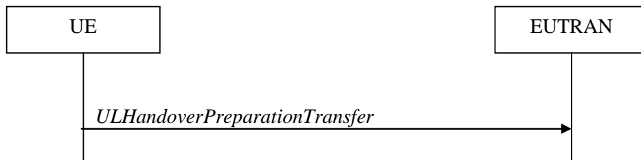
Figure 5.4.5.1-1: UL handover preparation transfer
