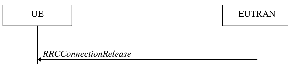
Figure 5.3.8.1-1: RRC connection release, successful
