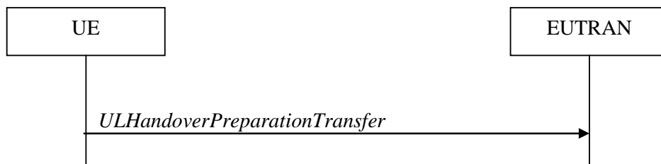
Figure 5.4.5.1-1: UL handover preparation transfer
