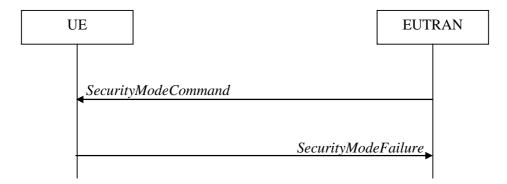
Figure 5.3.4.1-2: Security mode command, failure
