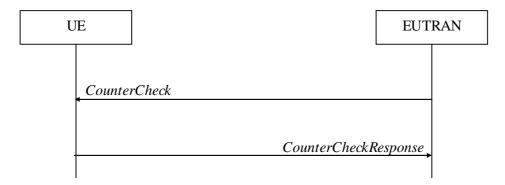
Figure 5.3.6.1-1: Counter check procedure
