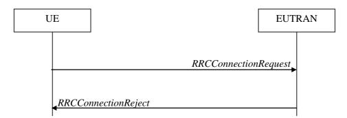
Figure 5.3.3.1-2: RRC connection establishment, network reject
