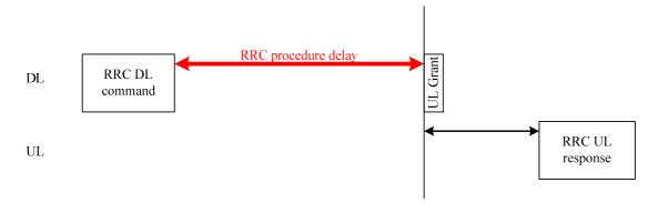
Figure 11.2-1: Illustration of RRC procedure delay
