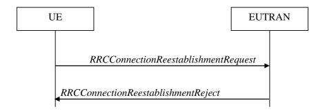
Figure 5.3.7.1-2: RRC connection re-establishment, failure
