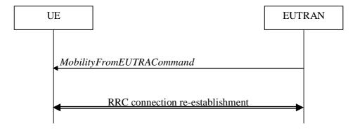
Figure 5.4.3.1-2: Mobility from E-UTRA, failure
