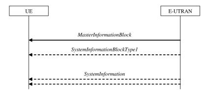
Figure 5.2.2.1-1: System information acquisition, normal
