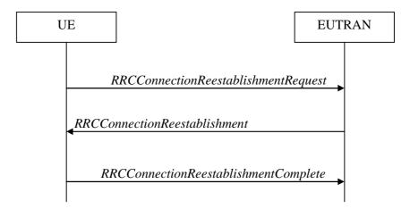
Figure 5.3.7.1-1: RRC connection re-establishment, successful
