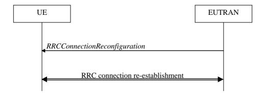
Figure 5.3.5.1-2: RRC connection reconfiguration, failure
