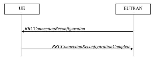
Figure 5.3.5.1-1: RRC connection reconfiguration, successful
