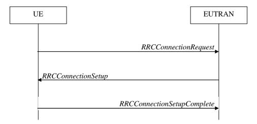
Figure 5.3.3.1-1: RRC connection establishment, successful
