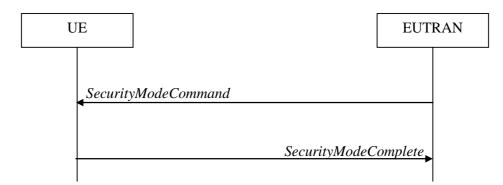
Figure 5.3.4.1-1: Security mode command, successful
