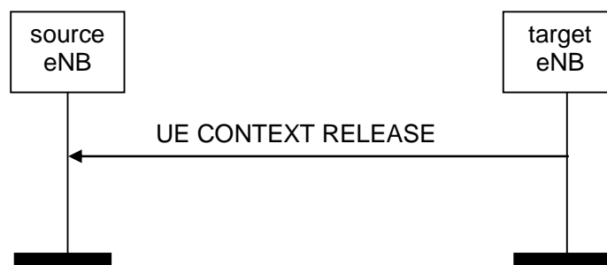
Figure 8.2.3.2-1: UE Context Release, successful operation for handover
