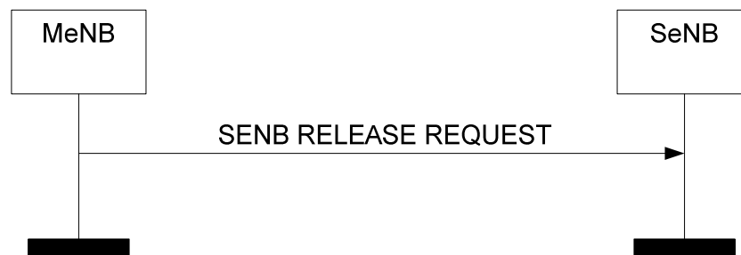
Figure 8.6.5.2-1: MeNB initiated SeNB Release, successful operation
