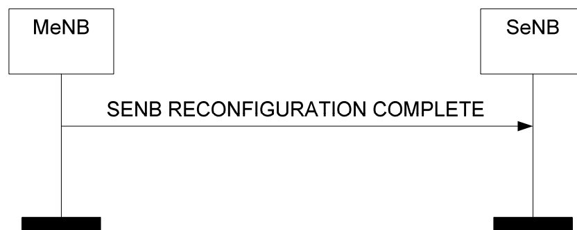
Figure 8.6.2.2-1: SeNB Reconfiguration Complete procedure, successful operation.
