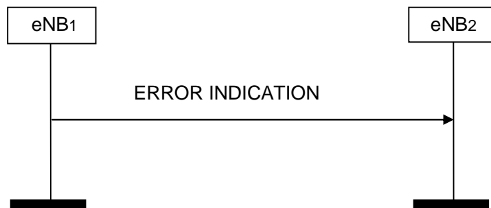
Figure 8.3.2.2-1: Error Indication, successful operation.
