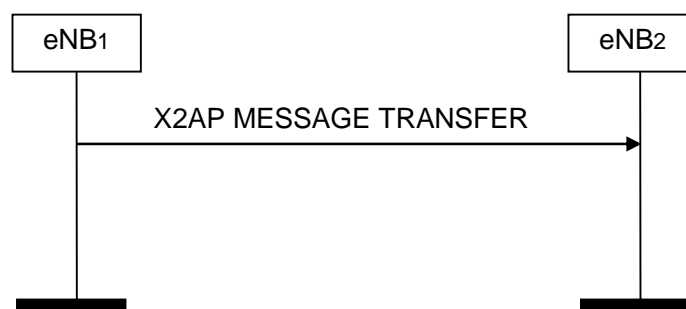
Figure 8.5.2-1: X2AP Message Transfer, successful operation
