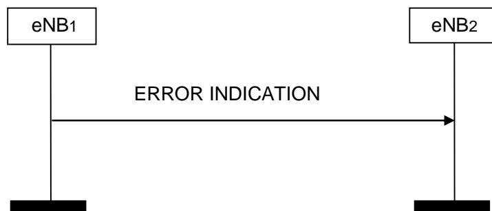
Figure 8.3.2.2-1: Error Indication, successful operation.
