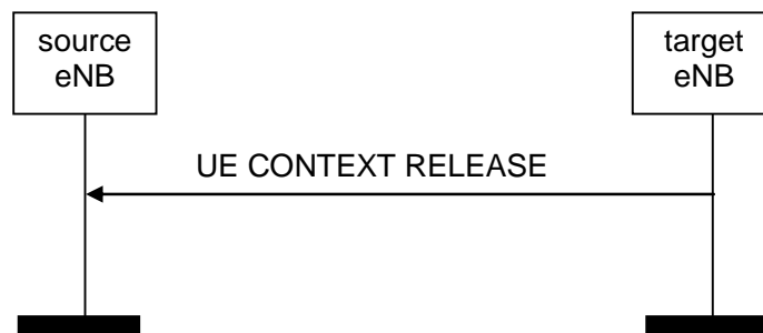
Figure 8.2.3.2-1: UE Context Release, successful operation for handover
