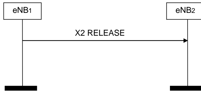
Figure 8.4.2-1: X2AP Release, successful operation
