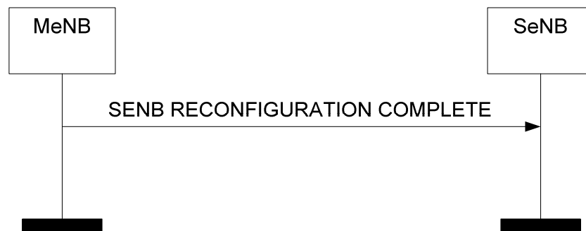
Figure 8.6.2.2-1: SeNB Reconfiguration Complete procedure, successful operation.
