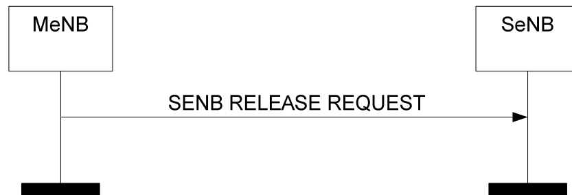
Figure 8.6.5.2-1: MeNB initiated SeNB Release, successful operation
