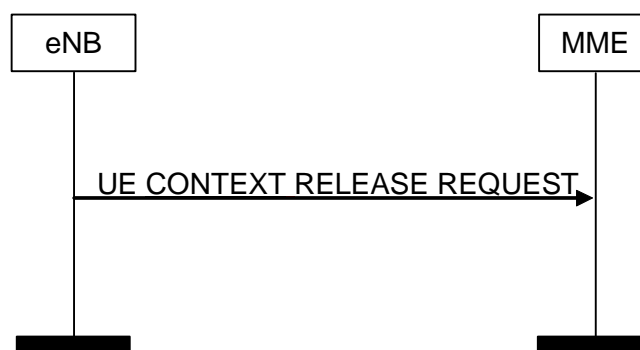
Figure 8.3.2.2-1: UE Context Release Request procedure. Successful operation.
