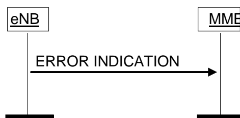
Figure 8.7.2.2-2: Error Indication procedure, eNB originated. Successful operation.
