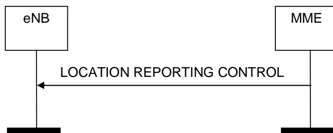
Figure 8.11.1.2-1: Location Reporting Control procedure. Successful operation.
