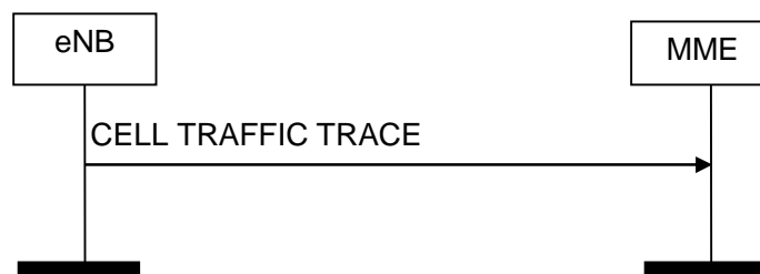
Figure 8.10.4.2-1: Cell Traffic Trace procedure. Successful operation.
