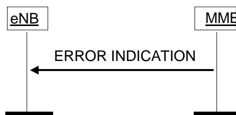
Figure 8.7.2.2-1: Error Indication procedure, MME originated. Successful operation.
