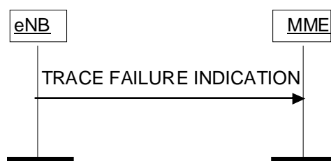
Figure 8.10.2.2-1: Trace Failure Indication procedure.
