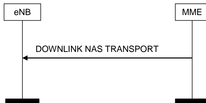
Figure 8.6.2.2-1: DOWNLINK NAS Transport Procedure
