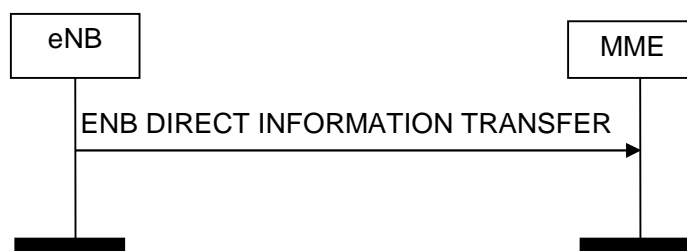
Figure 8.13.1.2-1: ENB Direct Information Transfer procedure. Successful operation.
