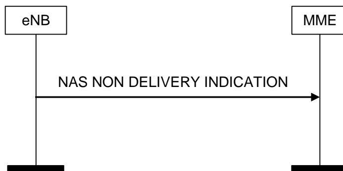
Figure 8.6.2.4-1: NAS NON DELIVERY INDICATION Procedure
