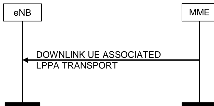
Figure 8.17.2.1-1: DOWNLINK UE ASSOCIATED LPPA Transport Procedure
