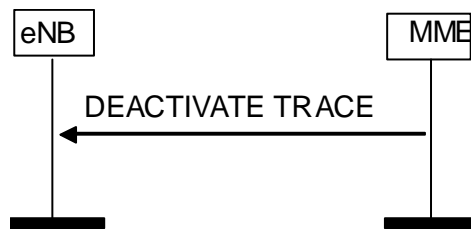
Figure 8.10.3.2-1: Deactivate Trace procedure. Successful operation.
