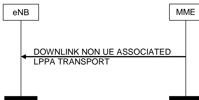
Figure 8.17.2.3-1: DOWNLINK NON UE ASSOCIATED LPPA Transport Procedure
