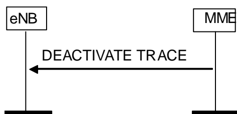
Figure 8.10.3.2-1: Deactivate Trace procedure. Successful operation.
