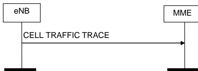
Figure 8.10.4.2-1: Cell Traffic Trace procedure. Successful operation.
