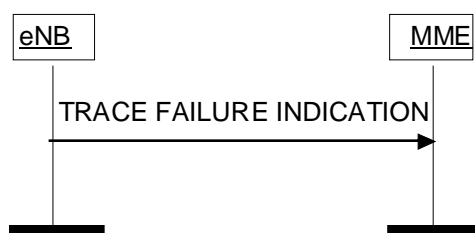
Figure 8.10.2.2-1: Trace Failure Indication procedure.
