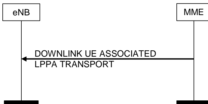
Figure 8.17.2.1-1: DOWNLINK UE ASSOCIATED LPPA Transport Procedure
