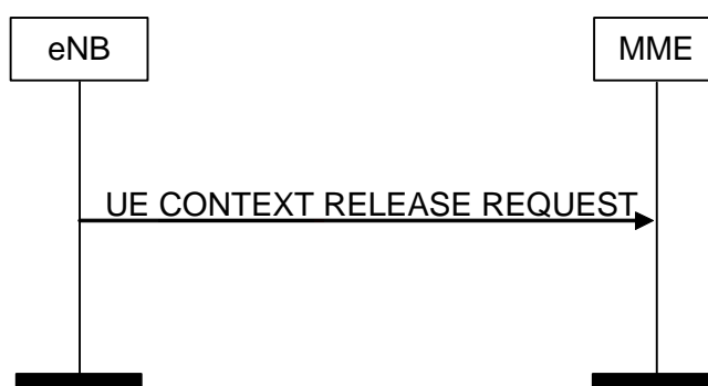
Figure 8.3.2.2-1: UE Context Release Request procedure. Successful operation.
