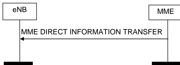
Figure 8.14.1.2-1: MME Direct Information Transfer procedure. Successful operation.
