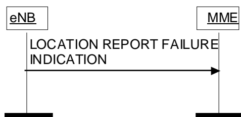
Figure 8.11.2.2-1: Location Report Failure Indication procedure.
