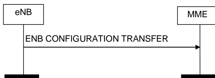
Figure 8.15.2.1-1: eNB Configuration Transfer procedure. Successful operation.
