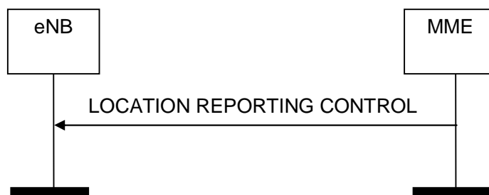
Figure 8.11.1.2-1: Location Reporting Control procedure. Successful operation.
