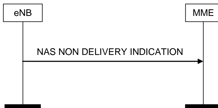
Figure 8.6.2.4-1: NAS NON DELIVERY INDICATION Procedure
