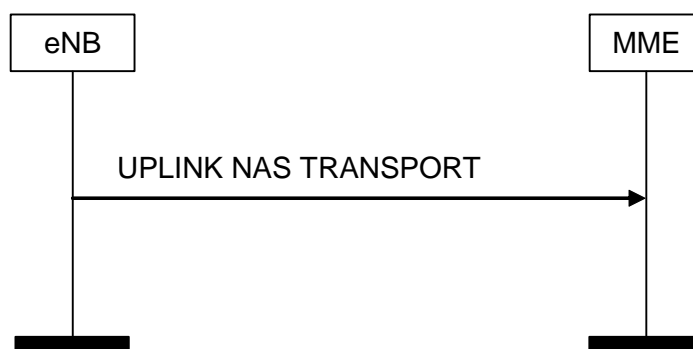
Figure 8.6.2.3-1: UPLINK NAS TRANSPORT Procedure
