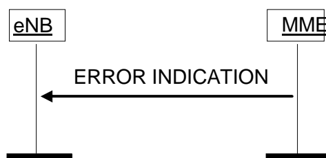
Figure 8.7.2.2-1: Error Indication procedure, MME originated. Successful operation.
