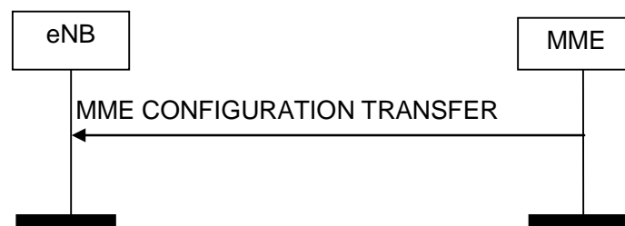
Figure 8.16.2.1-1: MME Configuration Transfer procedure. Successful operation.
