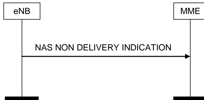
Figure 8.6.2.4-1: NAS NON DELIVERY INDICATION Procedure
