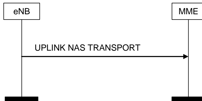
Figure 8.6.2.3-1: UPLINK NAS TRANSPORT Procedure
