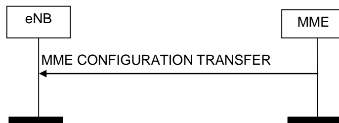
Figure 8.16.2.1-1: MME Configuration Transfer procedure. Successful operation.
