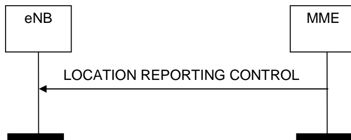
Figure 8.11.1.2-1: Location Reporting Control procedure. Successful operation.
