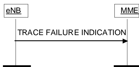
Figure 8.10.2.2-1: Trace Failure Indication procedure.
