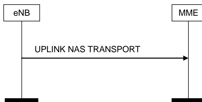
Figure 8.6.2.3-1: UPLINK NAS TRANSPORT Procedure
