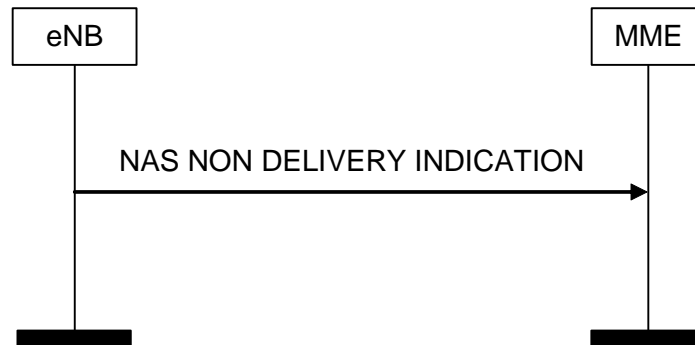
Figure 8.6.2.4-1: NAS NON DELIVERY INDICATION Procedure
