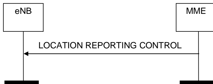
Figure 8.11.1.2-1: Location Reporting Control procedure. Successful operation.
