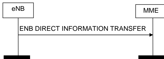
Figure 8.13.1.2-1: ENB Direct Information Transfer procedure. Successful operation.
