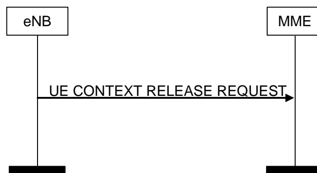
Figure 8.3.2.2-1: UE Context Release Request procedure. Successful operation.
