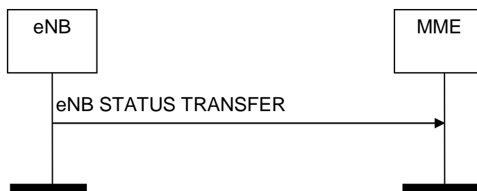
Figure 8.4.6.2-1: eNB Status Transfer procedure
