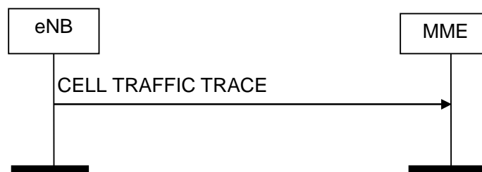
Figure 8.10.4.2-1: Cell Traffic Trace procedure. Successful operation.
