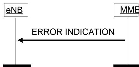
Figure 8.7.2.2-1: Error Indication procedure, MME originated. Successful operation.
