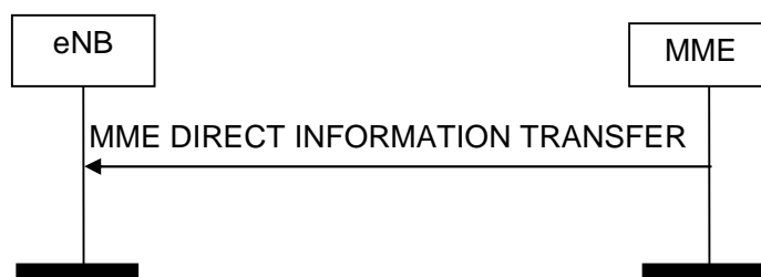
Figure 8.14.1.2-1: MME Direct Information Transfer procedure. Successful operation.
