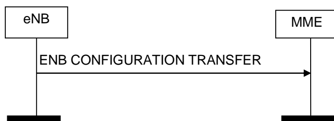
Figure 8.15.2.1-1: eNB Configuration Transfer procedure. Successful operation.
