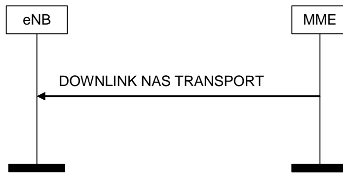
Figure 8.6.2.2-1: DOWNLINK NAS Transport Procedure
