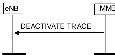
Figure 8.10.3.2-1: Deactivate Trace procedure. Successful operation.
