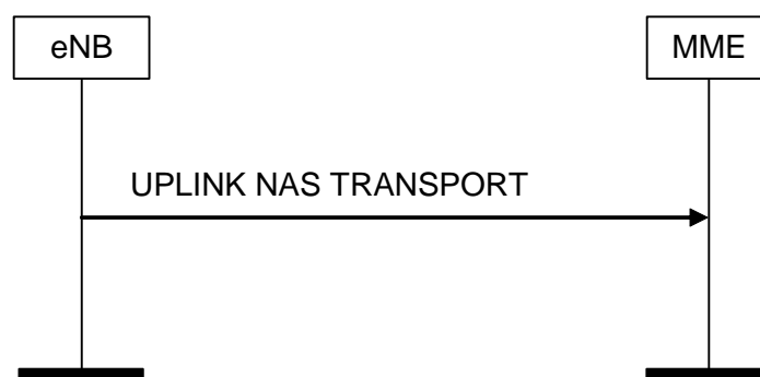
Figure 8.6.2.3-1: UPLINK NAS TRANSPORT Procedure
