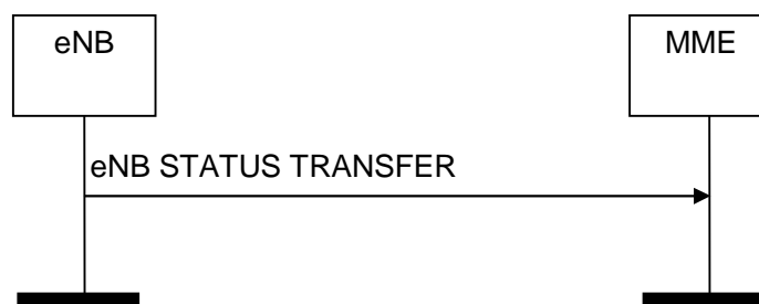
Figure 8.4.6.2-1: eNB Status Transfer procedure
