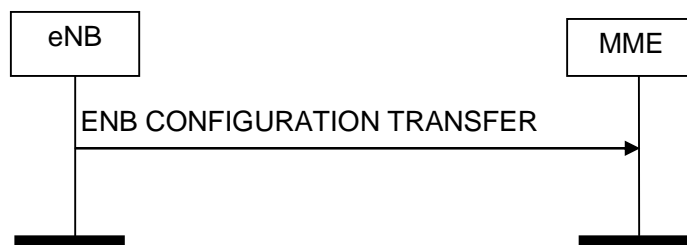
Figure 8.15.2.1-1: eNB Configuration Transfer procedure. Successful operation.
