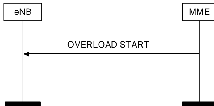
Figure 8.7.6.2-1: Overload Start procedure
