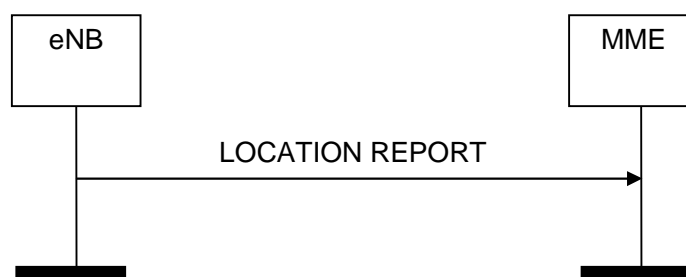
Figure 8.11.3.2-1: Location Report procedure. Successful operation.
