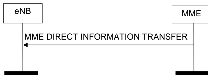
Figure 8.14.1.2-1: MME Direct Information Transfer procedure. Successful operation.
