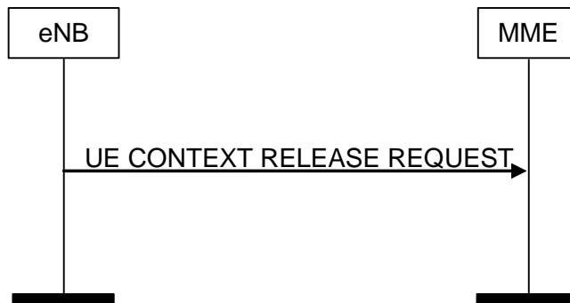
Figure 8.3.2.2-1: UE Context Release Request procedure. Successful operation.
