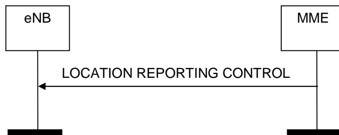
Figure 8.11.1.2-1: Location Reporting Control procedure. Successful operation.
