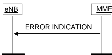
Figure 8.7.2.2-1: Error Indication procedure, MME originated. Successful operation.
