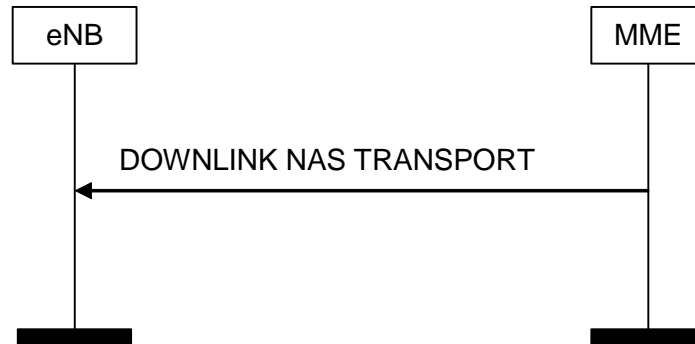
Figure 8.6.2.2-1: DOWNLINK NAS Transport Procedure
