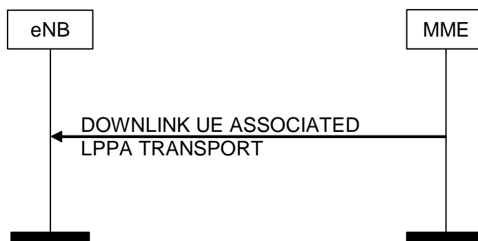
Figure 8.17.2.1-1: DOWNLINK UE ASSOCIATED LPPA Transport Procedure
