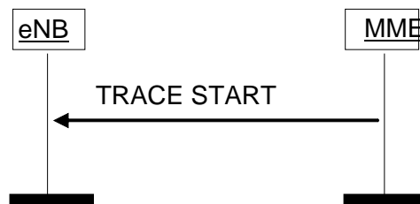
Figure 8.10.1.2-1: Trace Start procedure.
