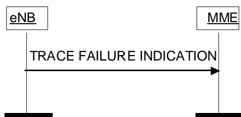
Figure 8.10.2.2-1: Trace Failure Indication procedure.
