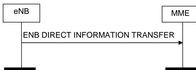
Figure 8.13.1.2-1: ENB Direct Information Transfer procedure. Successful operation.
