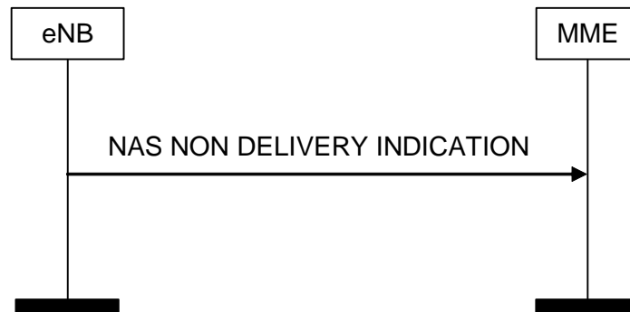
Figure 8.6.2.4-1: NAS NON DELIVERY INDICATION Procedure
