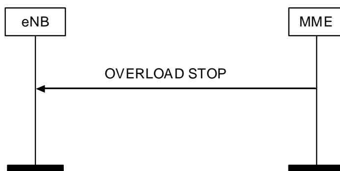
Figure 8.7.7.2.-1: Overload Stop procedure
