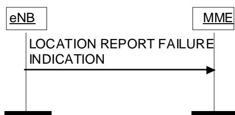
Figure 8.11.2.2-1: Location Report Failure Indication procedure.
