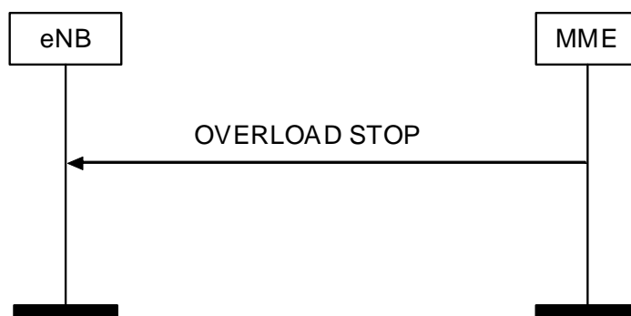
Figure 8.7.7.2.-1: Overload Stop procedure
