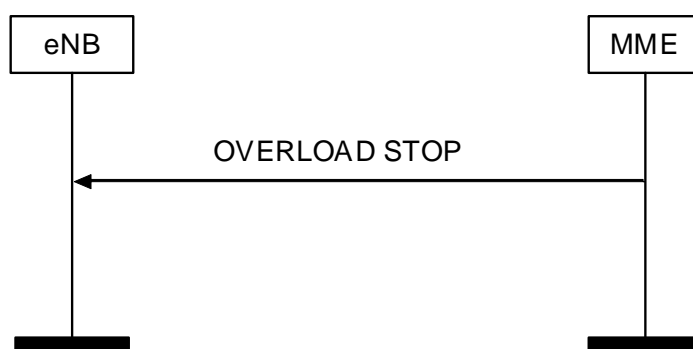
Figure 8.7.7.2.-1: Overload Stop procedure
