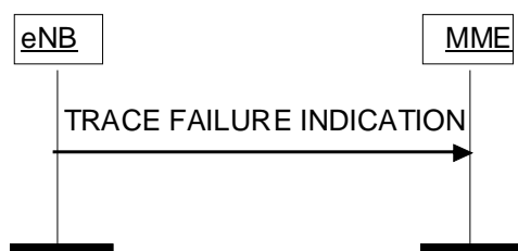
Figure 8.10.2.2-1: Trace Failure Indication procedure.
