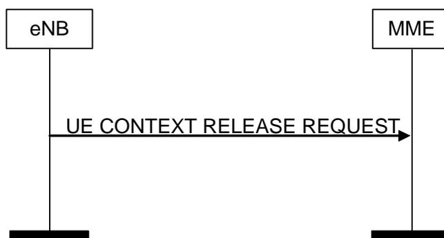
**Figure 8.3.2.2-1: UE Context Release Request procedure. Successful operation.**
