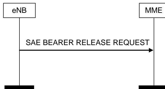
**Figure 8.2.3.2.2-1: SAE Bearer Release Request procedure. Successful operation.**
