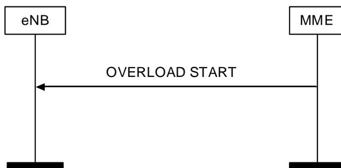
**Figure 8.7.6.2-1: Overload Start procedure**
