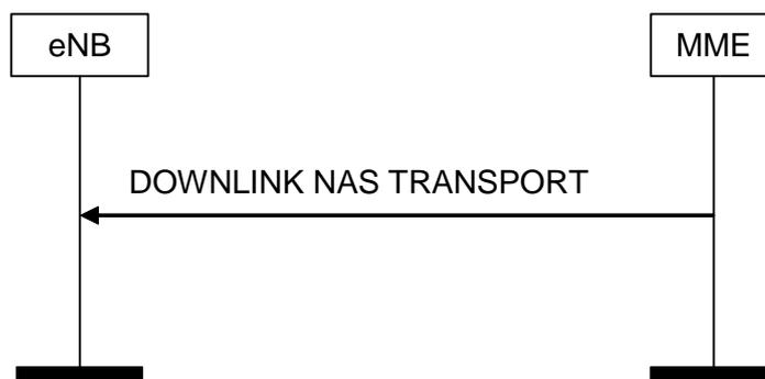
**Figure 8.6.2.2-1: DOWNLINK NAS Transport Procedure**
