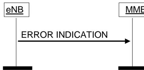
**Figure 8.7.2.2-2: Error Indication procedure, eNB originated. Successful operation.**
