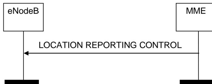
**Figure 8.11.1.2-1: Location Reporting Control procedure. Successful operation.**
