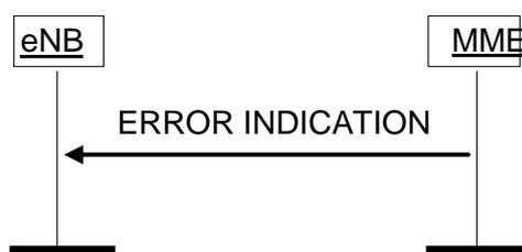
Figure 8.7.2.2-1: Error Indication procedure, MME originated. Successful operation.
