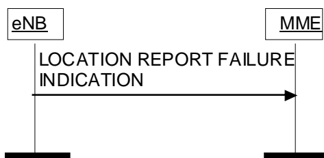
Figure 8.11.2.2-1: Location Report Failure Indication procedure.
