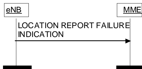
Figure 8.11.2.2-1: Location Report Failure Indication procedure.
