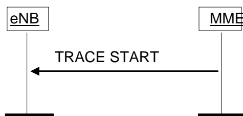
Figure 8.10.1.2-1: Trace Start procedure.
