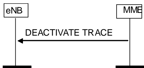
Figure 8.10.3.2-1: Deactivate Trace procedure. Successful operation.
