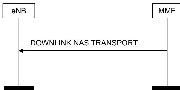
Figure 8.6.2.2-1: DOWNLINK NAS Transport Procedure
