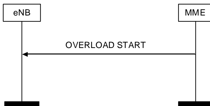
Figure 8.7.6.2-1: Overload Start procedure
