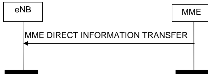
Figure 8.14.1.2-1: MME Direct Information Transfer procedure. Successful operation.
