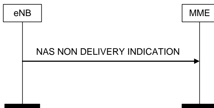
Figure 8.6.2.4-1: NAS NON DELIVERY INDICATION Procedure
