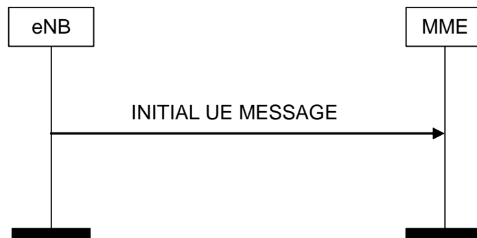
Figure 8.6.2.1-1: Initial UE Message procedure
