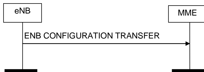
Figure 8.15.2.1-1: eNB Configuration Transfer procedure. Successful operation.
