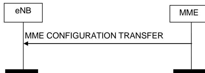
Figure 8.16.2.1-1: MME Configuration Transfer procedure. Successful operation.
