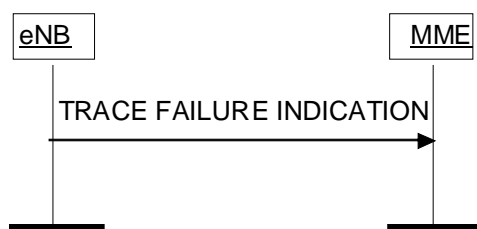
Figure 8.10.2.2-1: Trace Failure Indication procedure.
