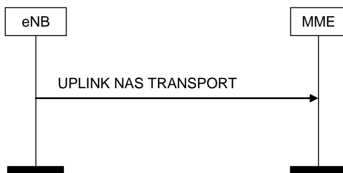
Figure 8.6.2.3-1: UPLINK NAS TRANSPORT Procedure
