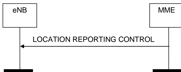
Figure 8.11.1.2-1: Location Reporting Control procedure. Successful operation.
