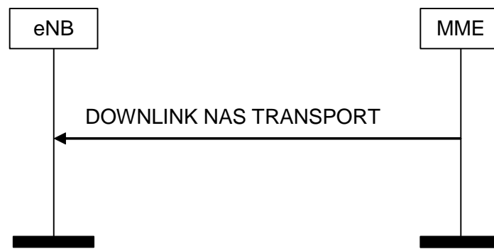
Figure 8.6.2.2-1: DOWNLINK NAS Transport Procedure
