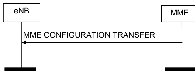
Figure 8.16.2.1-1: MME Configuration Transfer procedure. Successful operation.
