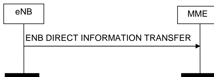
Figure 8.13.1.2-1: ENB Direct Information Transfer procedure. Successful operation.
