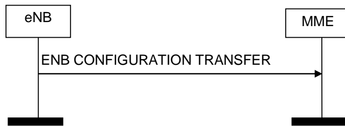
Figure 8.15.2.1-1: eNB Configuration Transfer procedure. Successful operation.
