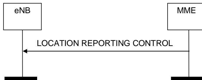
Figure 8.11.1.2-1: Location Reporting Control procedure. Successful operation.
