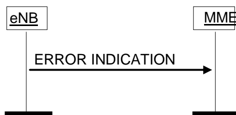
Figure 8.7.2.2-2: Error Indication procedure, eNB originated. Successful operation.
