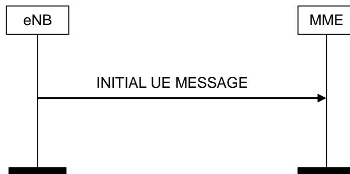
Figure 8.6.2.1-1: Initial UE Message procedure
