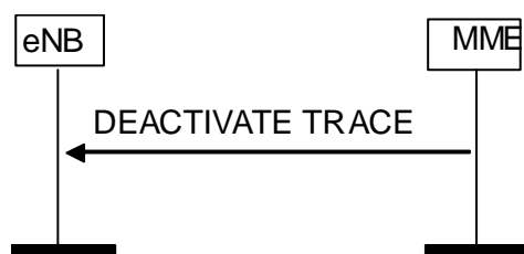
Figure 8.10.3.2-1: Deactivate Trace procedure. Successful operation.
