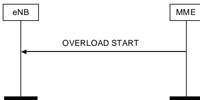
Figure 8.7.6.2-1: Overload Start procedure
