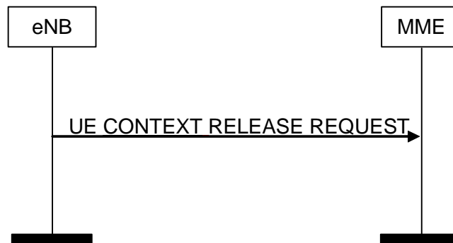
Figure 8.3.2.2-1: UE Context Release Request procedure. Successful operation.
