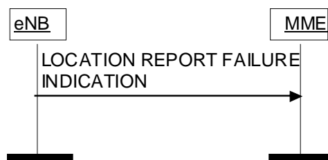
Figure 8.11.2.2-1: Location Report Failure Indication procedure.
