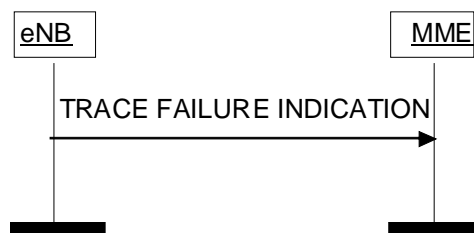
Figure 8.10.2.2-1: Trace Failure Indication procedure.
