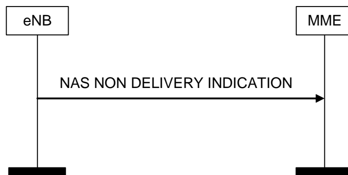
Figure 8.6.2.4-1: NAS NON DELIVERY INDICATION Procedure
