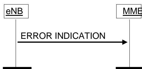
Figure 8.7.2.2-2: Error Indication procedure, eNB originated. Successful operation.
