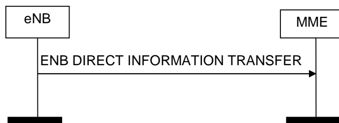
Figure 8.13.1.2-1: ENB Direct Information Transfer procedure. Successful operation.
