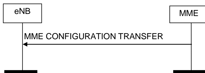
Figure 8.16.2.1-1: MME Configuration Transfer procedure. Successful operation.
