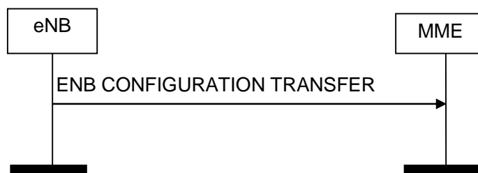
Figure 8.15.2.1-1: eNB Configuration Transfer procedure. Successful operation.
