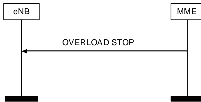
Figure 8.7.7.2.-1: Overload Stop procedure
