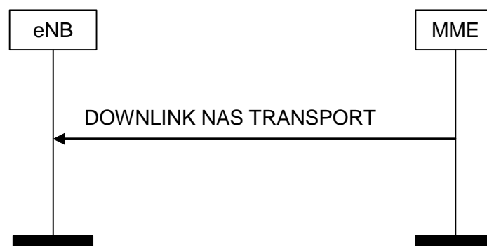
Figure 8.6.2.2-1: DOWNLINK NAS Transport Procedure
