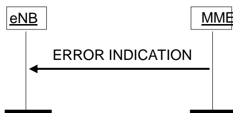
Figure 8.7.2.2-1: Error Indication procedure, MME originated. Successful operation.
