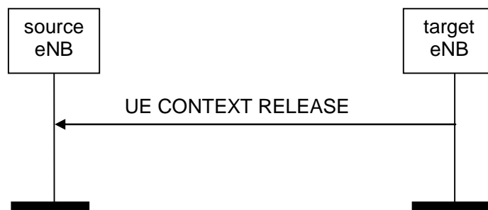
Figure 8.2.3.2-1: UE Context Release, successful operation
