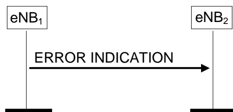
Figure 8.3.2.2-1: Error Indication, successful operation.
