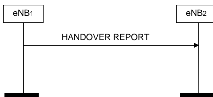
Figure 8.3.10.2-1: Handover Report, successful operation
