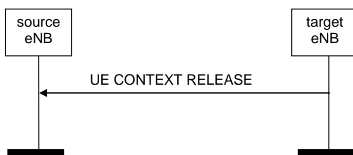
Figure 8.2.3.2-1: UE Context Release, successful operation
