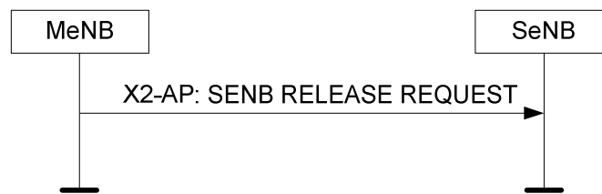
Figure 8.6.5.2-1: MeNB initiated SeNB Release, successful operation
