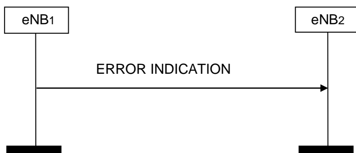
Figure 8.3.2.2-1: Error Indication, successful operation.
