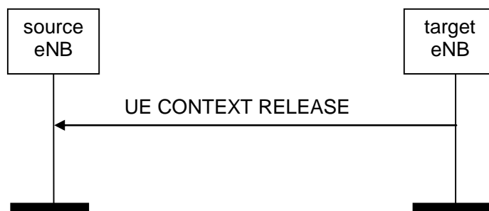
Figure 8.2.3.2-1: UE Context Release, successful operation for handover
