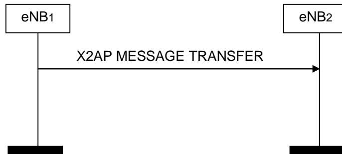
Figure 8.5.2-1: X2AP Message Transfer, successful operation
