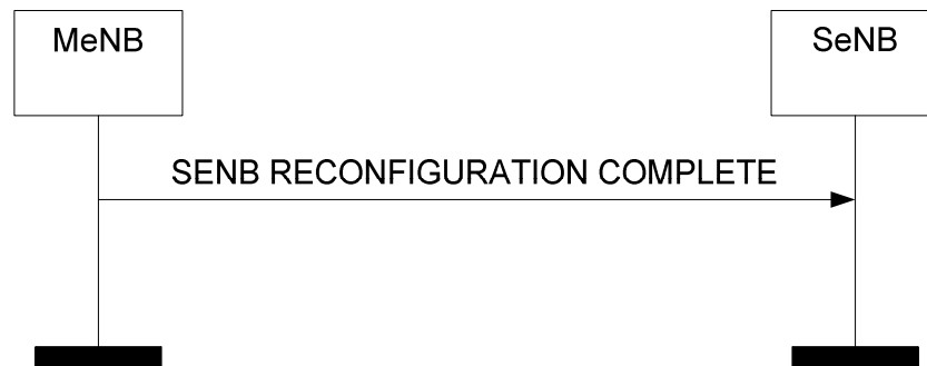
Figure 8.6.2.2-1: SeNB Reconfiguration Complete procedure, successful operation.
