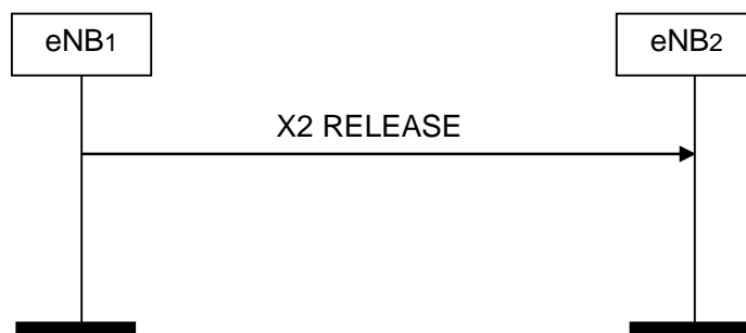
Figure 8.4.2-1: X2AP Release, successful operation
