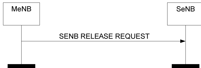
Figure 8.6.5.2-1: MeNB initiated SeNB Release, successful operation
