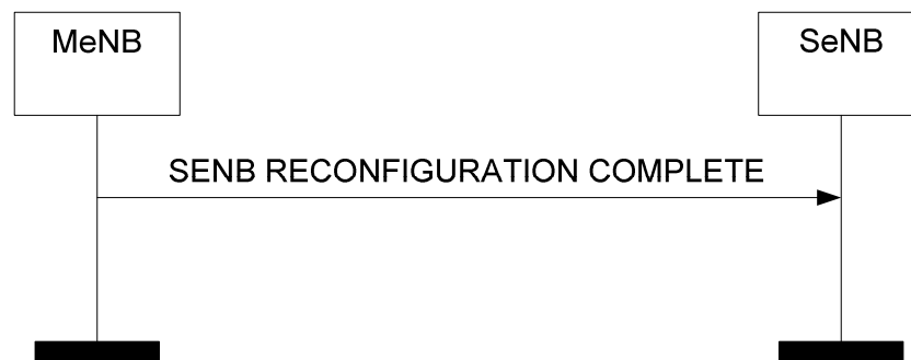
Figure 8.6.2.2-1: SeNB Reconfiguration Complete procedure, successful operation.
