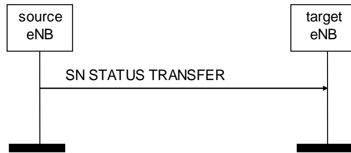
Figure 8.2.2.2-1: SN Status Transfer, successful operation
