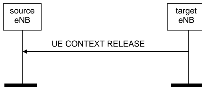
Figure 8.2.3.2-1: UE Context Release, successful operation for handover
