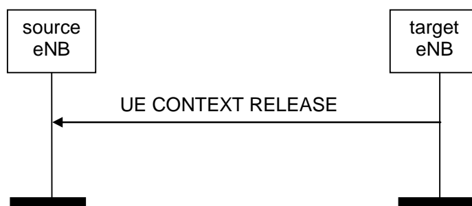
Figure 8.2.3.2-1: UE Context Release, successful operation
