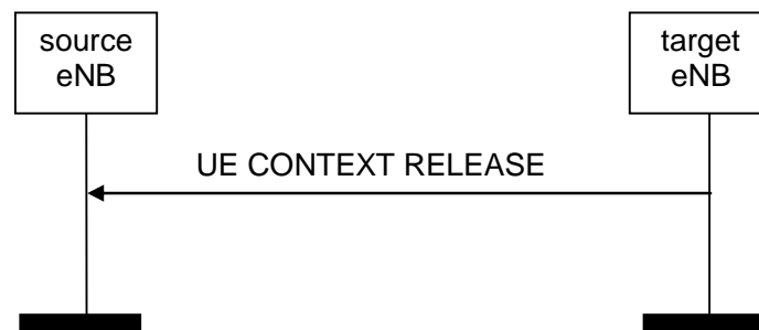
Figure 8.2.3.2-1: UE Context Release, successful operation
