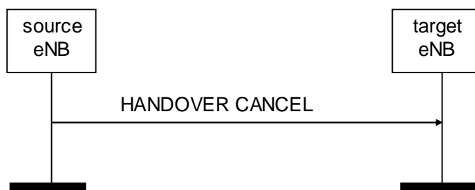
Figure 8.2.4.2-1: Handover Cancel, successful operation
