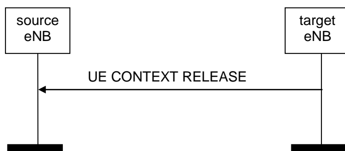
Figure 8.2.3.2-1: UE Context Release, successful operation
