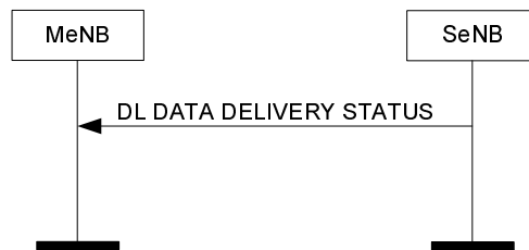
Figure 5.4.2.1-1: Successful Downlink Data Delivery Status
