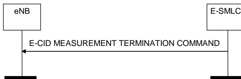
Figure 8.2.4.2-1: E-CID Measurement Reporting Control procedure.
