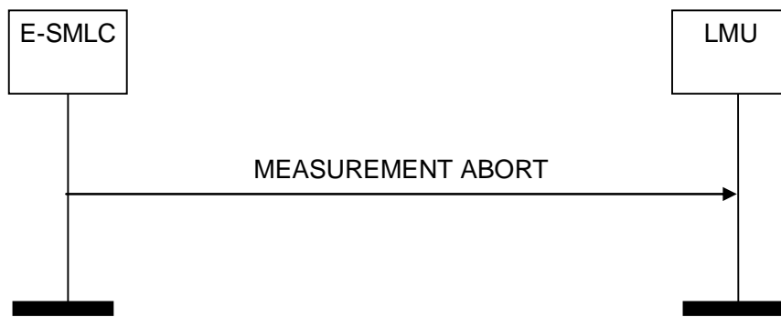
Figure 8.2.3.2.1: Measurement Abort Procedure: Successful Operation.
