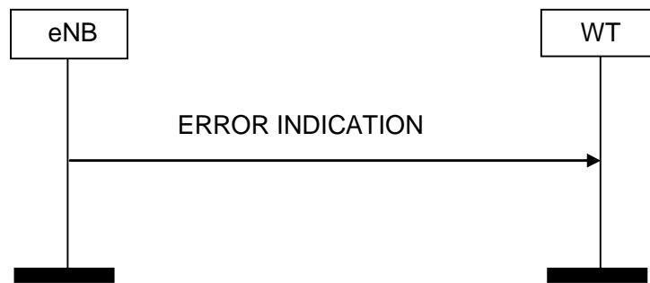
Figure 8.6.2-1: Error Indication procedure, eNB originated. Successful operation.
