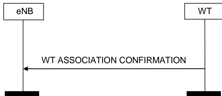
Figure 8.13.2-1: WT Association Confirm procedure, successful operation
