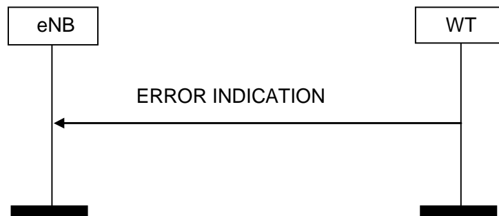
Figure 8.6.2-2: Error Indication procedure, WT originated. Successful operation.
