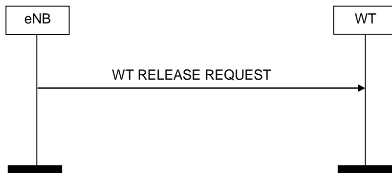
Figure 8.11.2-1: eNB initiated WT Release, successful operation
