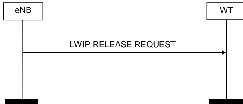
Figure 8.16.2-1: eNB initiated LWIP Release, successful operation
