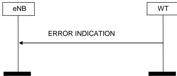
Figure 8.6.2-2: Error Indication procedure, WT originated. Successful operation.
