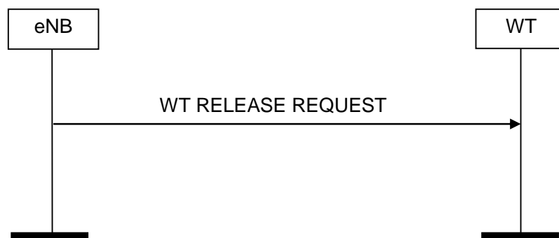
Figure 8.11.2-1: eNB initiated WT Release, successful operation
