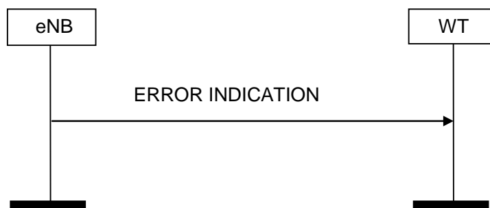
Figure 8.6.2-1: Error Indication procedure, eNB originated. Successful operation.
