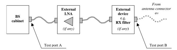
Figure 4.10.2-1: Receiver test ports
