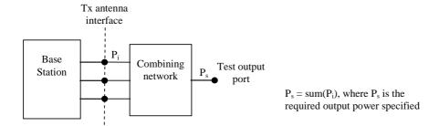
Figure 4.10.7.2-1: Transmitter test set-up
