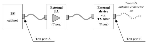
Figure 4.10.1-1: Transmitter test ports
