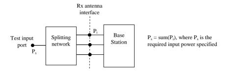
Figure 4.10.7.1-1: Receiver test set-up
