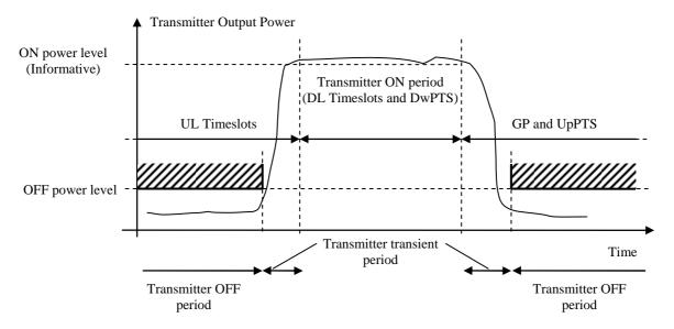
Figure 6.4.1-1: Illustration of the relations of transmitter ON period, transmitter OFF period and transmitter transient period
