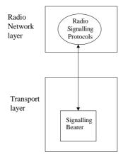
Figure 8: Separation of Radio Network Protocols and transport over the lur-g interface
