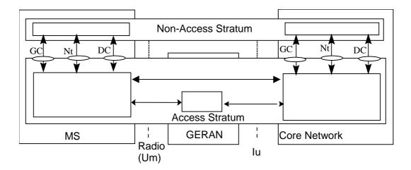
Figure 2: UMTS Architecture applied to GERAN
