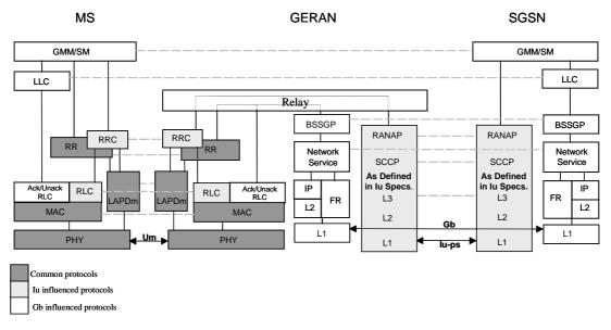
Figure 5: Control Plane protocols towards Packet Switched Core Network domain
