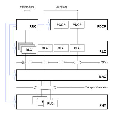
Figure 11: Radio Interface protocol architecture with FLO
