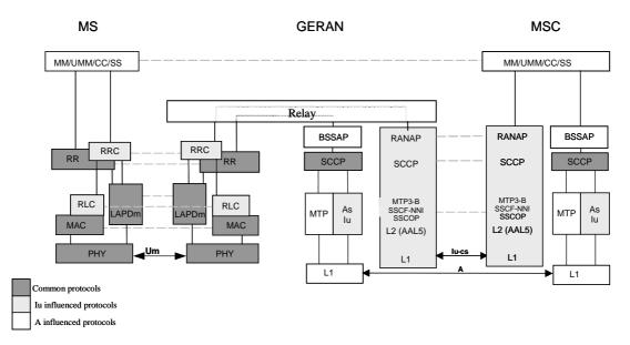
Figure 7: Control Plane Protocols towards Circuit-Switched Core Network Domain
