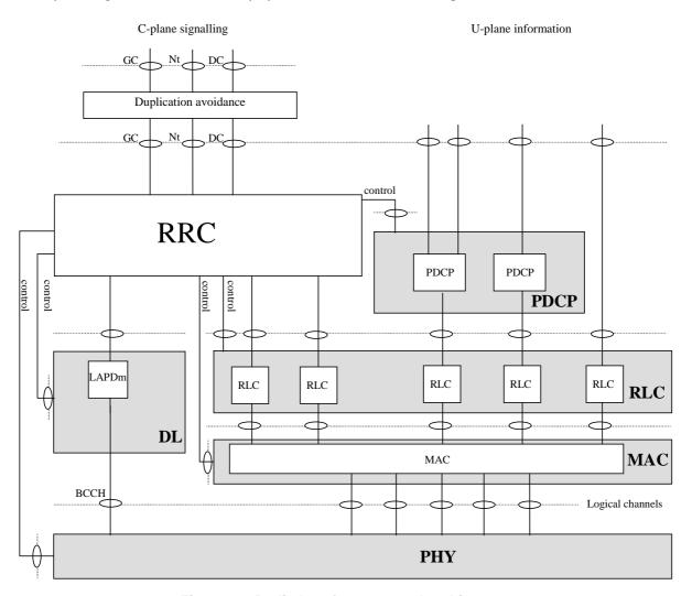
Figure 10: Radio Interface protocol architecture
