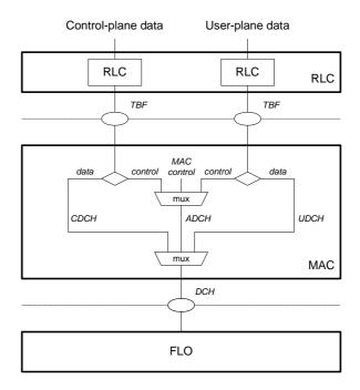
**Figure 14: Logical Channels and Transport Channels**
