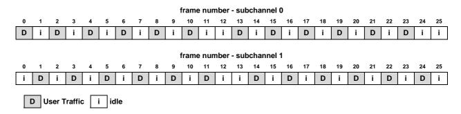
Figure 16: SBPSCH/H - Multiframe mapping of logical channels
