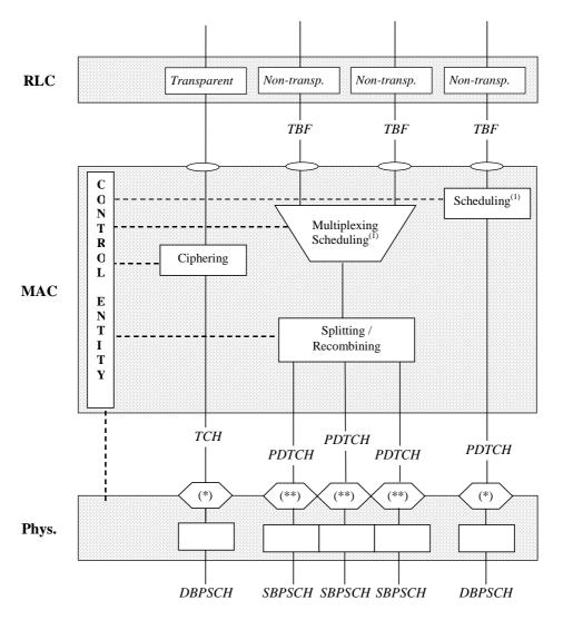
Figure 13. Example of MAC functions for one user (MS side – user plane)
