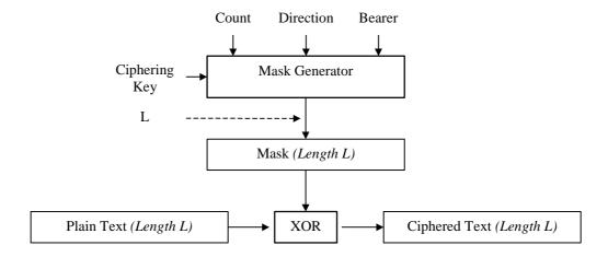
Figure 17: Ciphering Principle
