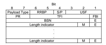
Figure B.1: Downlink RLC/MAC Data Block header (CS-1, CS-2, CS-3, CS-4)
