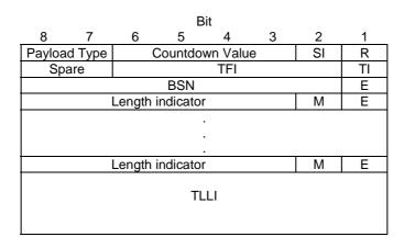
Figure B.2: Uplink RLC/MAC Data Block Header (CS-1, CS-2, CS-3 and CS-4)
