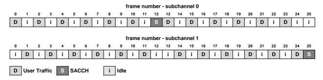
Figure 14: DBPSCH/H - Multiframe mapping of logical channels
