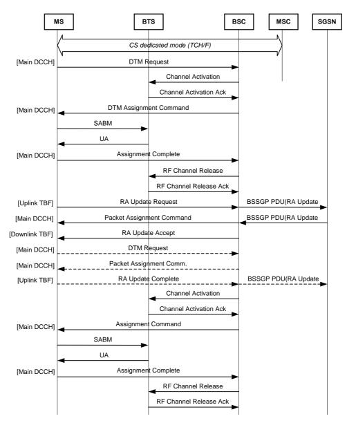
Figure 15: Routeing Area Update procedure in dedicated mode, packet idle mode and Ready state; performed on TBFs
