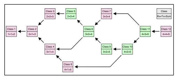
Figure 19 - Incremental support of multislot classes.
