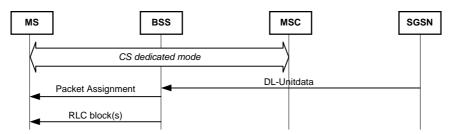
Figure 7: Example of a successful establishment of a PS MT session while in dedicated mode, packet idle mode and Ready state
