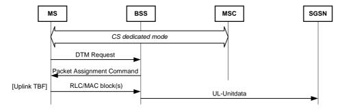
Figure 13: Cell Update procedure in dedicated mode, packet idle mode and Ready state; performed ion a TBF
