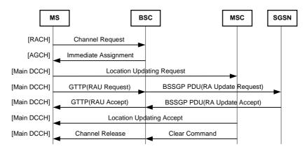
Figure 17: Parallel LA and RA Update procedures: the RAU finishes first
