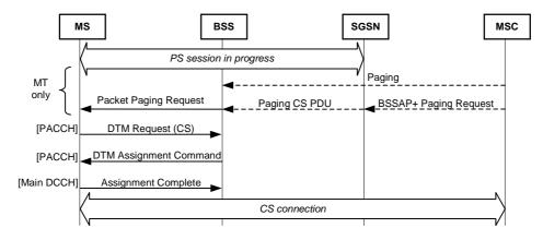
Figure 10: Successful establishment of a CS connection while in packet transfer mode without interruption of the packet session
