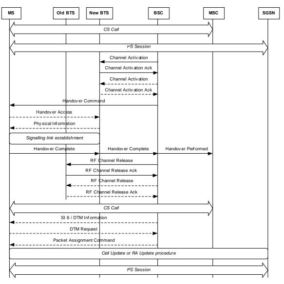
Figure 11: Successful internal, dual handover procedure
