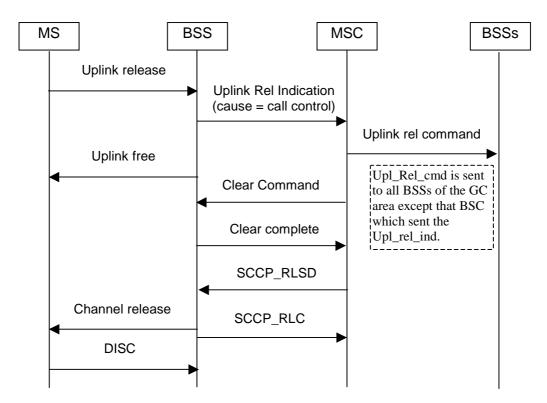
NOTE: The messages CLEAR CMD, CLEAR COM, etc., are used to release the dedicated connection of the talker.
