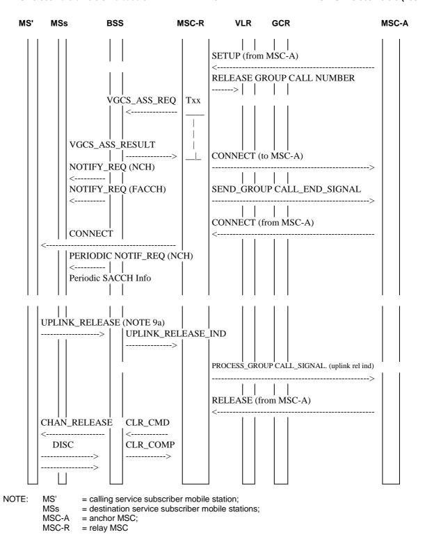
Figure 3: Signalling information required for establishing voice group calls by a service subscriber roaming in the relay MSC area
