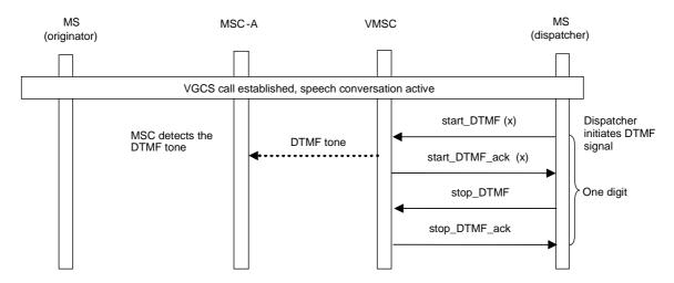
Figure 7c: Signalling required for communication of DTMF digit entry by an entitled mobile dispatcher, if the mobile dispatcher is controlled by a visited MSC (could be a relay MSC) of the group call.
