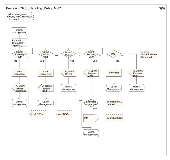
Figure 10: The VGCS handling process in the relay MSC (sheet 5 of 6)
