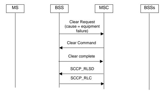
NOTE: The messages CLEAR CMD, CLEAR COM, etc., are used to release the radio and terrestrial resources for the cell not serving the talker. The same message flow applies also for all other cause values.
