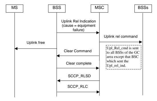
NOTE: The messages CLEAR CMD, CLEAR COM, etc., are used to release the radio and terrestrial resources for the cell serving the talker. The same message flow applies for all cause values different from "call control", and "radio interface failure".
