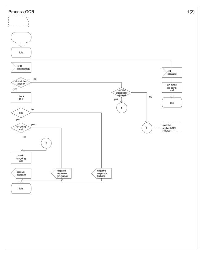
Figure 11: The process in the GCR (sheet 1 of 2)
