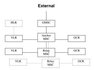
Figure 1: Functional architecture with a Group Call Register
