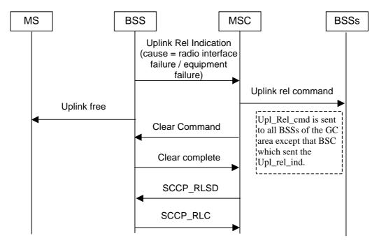
NOTE: The messages CLEAR CMD, CLEAR COM, etc., are used to release the dedicated connection of the talker. The same message flow applies for all cause values different from "call control".
