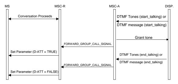
Figure 5b: Signalling information required when the talker is attached to a Relay MSC and a dispatcher wishes to speak
