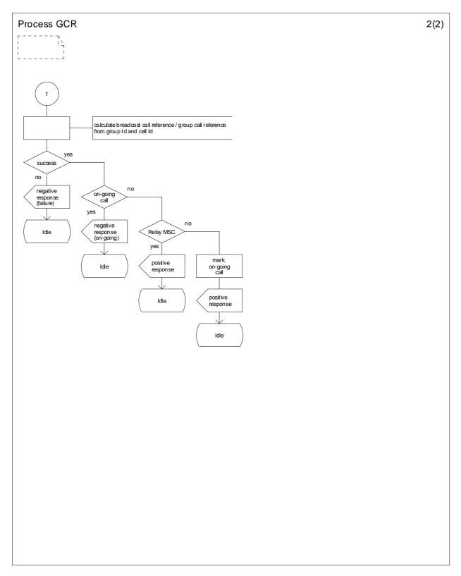
Figure 11: The process in the GCR (sheet 2 of 2)
