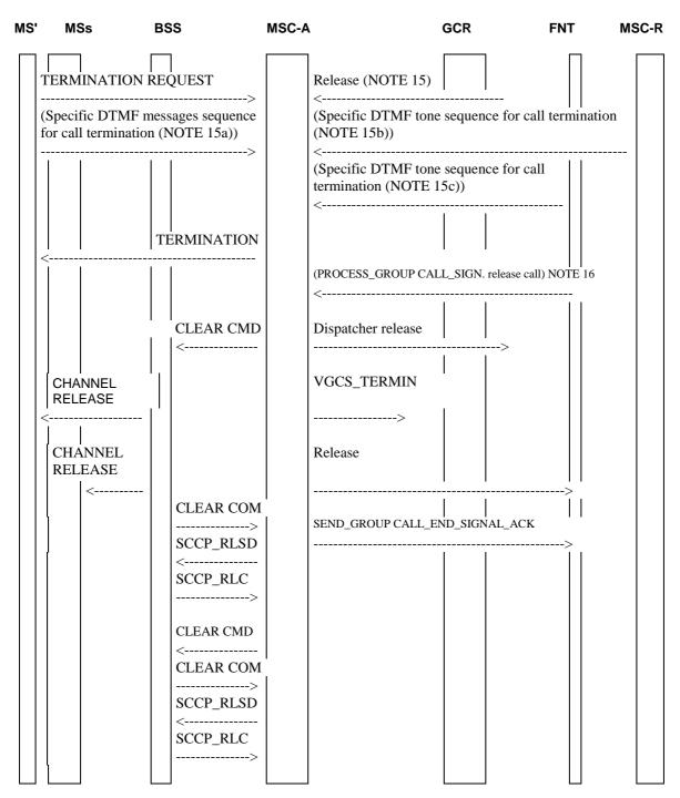
Figure 7: Signalling required to disconnect the group call
