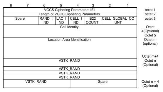
Figure 10.5.2.42b.1: VGCS Ciphering Parameters Information Element
