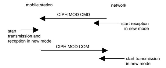
Figure 3.4.7.2.1: Ciphering mode setting sequence
