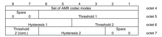
Figure 10.5.2.21aa.4: Parameters for multirate speech field for the Multirate speech versions 1 & 2 when a set of three codec modes is chosen
