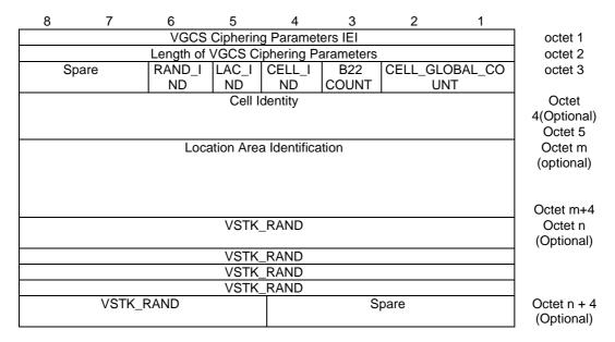
Figure 10.5.2.42b.1: VGCS Ciphering Parameters Information Element
