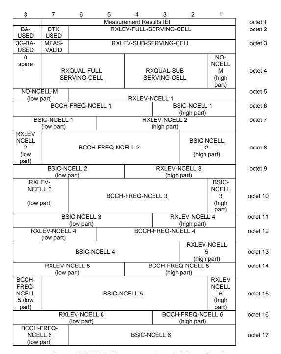
Figure 10.5.2.20.1: Measurement Results information element
