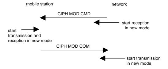
Figure 3.4.7.2.1: Ciphering mode setting sequence
