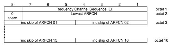
Figure 10.5.2.12.1: Frequency Channel Sequence information element
