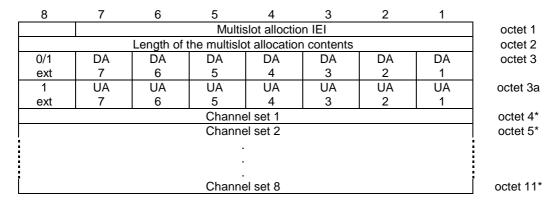
Figure 10.5.2.21b.1: Multislot Allocation information element
