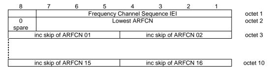
Figure 10.5.2.12.1: Frequency Channel Sequence information element
