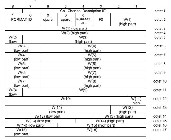
Figure 10.5.2.1b.3.1: *Cell Channel Description* information element (1024 range format)
