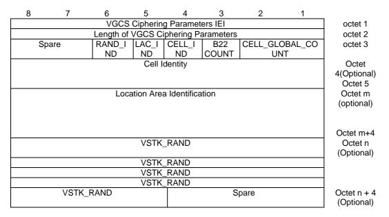
Figure 10.5.2.42b.1: VGCS Ciphering Parameters Information Element
