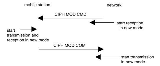
Figure 3.4.7.2.1: Ciphering mode setting sequence
