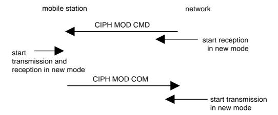
Figure 3.4.7.2.1: Ciphering mode setting sequence
