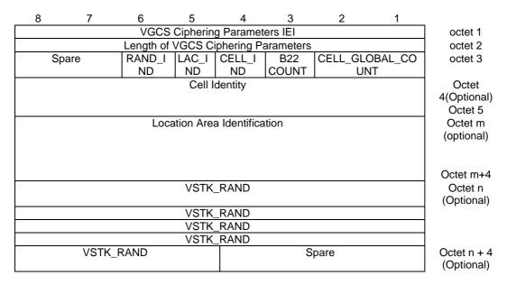
Figure 10.5.2.42b.1: VGCS Ciphering Parameters Information Element
