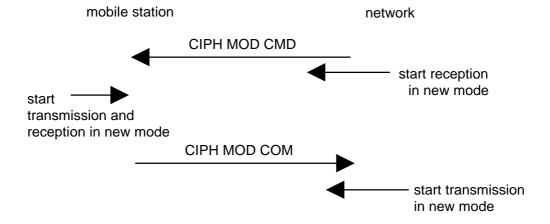
Figure 3.4.7.2.1: Ciphering mode setting sequence
