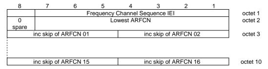
Figure 10.5.2.12.1: Frequency Channel Sequence information element
