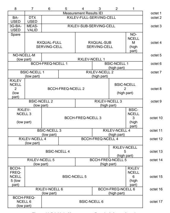
Figure 10.5.2.20.1: Measurement Results information element
