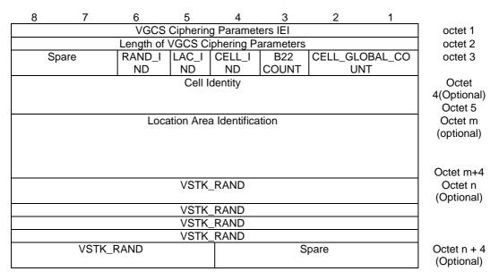
Figure 10.5.2.42b.1: VGCS Ciphering Parameters Information Element
