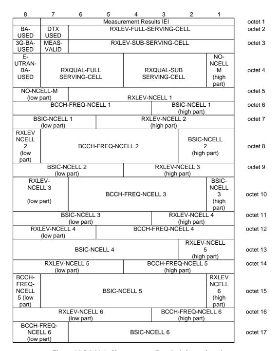
Figure 10.5.2.20.1: Measurement Results information element
