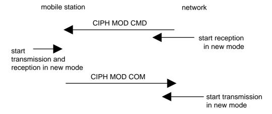
Figure 3.4.7.2.1: Ciphering mode setting sequence
