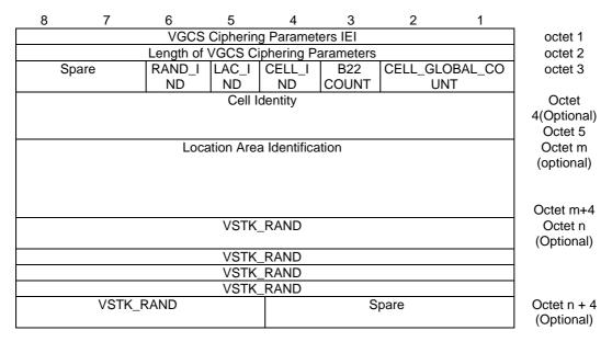
Figure 10.5.2.42b.1: VGCS Ciphering Parameters Information Element
