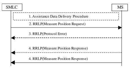
Figure 2.1: Position Measurement procedure
