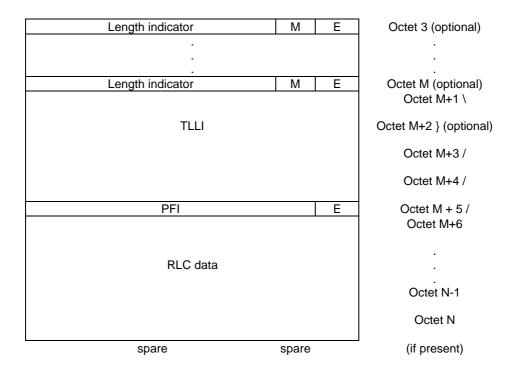
NOTE: The field mapping convention for GPRS (sub-clause 10.0b.3.1) applies. According to that, in particular regarding the TLLI field, the *most significant byte* of the TLLI value shall be mapped on octet M+1 and the *least significant byte* of the TLLI value shall be mapped on octet M+4 of the uplink RLC data block.
