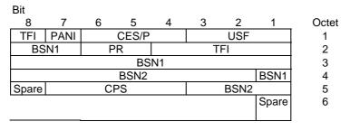
Figure 10.3a.3.7.1: Combined downlink RLC data block header for DBS-7 and DBS-8.
