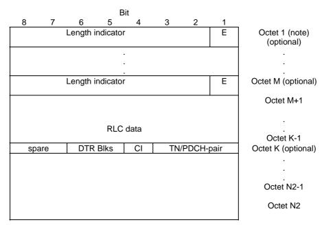
NOTE: If padding is used, then "Octet 1" shall be replaced by "Octet 7", see example in annex J.
