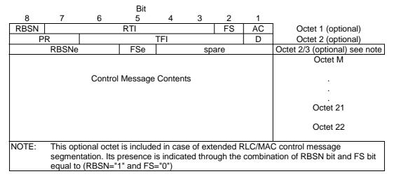
Figure 10.3.1.2: Downlink RLC/MAC control block message contents
